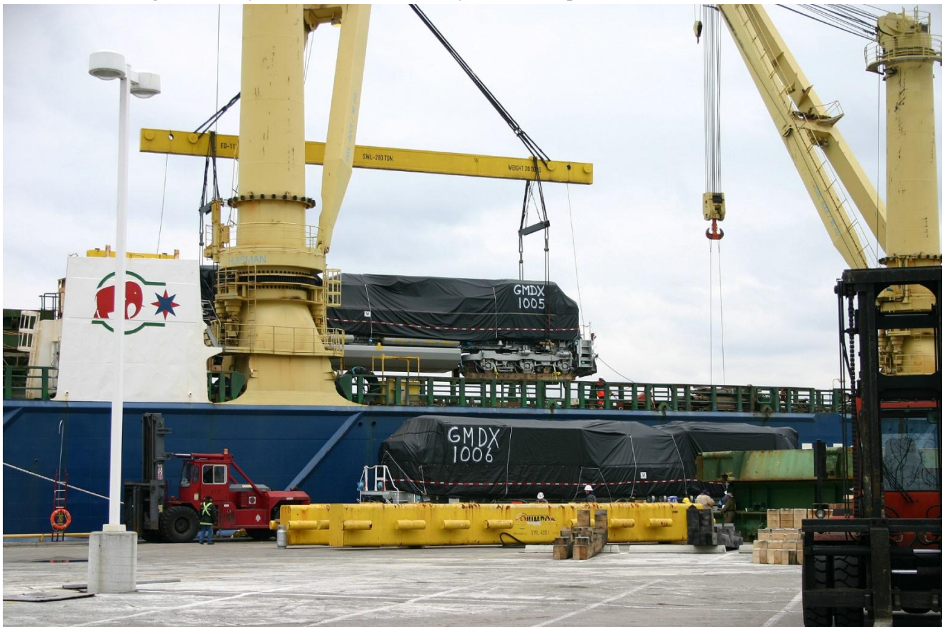
GMDX1005 being lowered into the hold of MV Jumbo Vision on 27th November with GMDX1006 still on the wharf note the wooden bogie brackets to be fitted before loading. Photo Joe Zika
