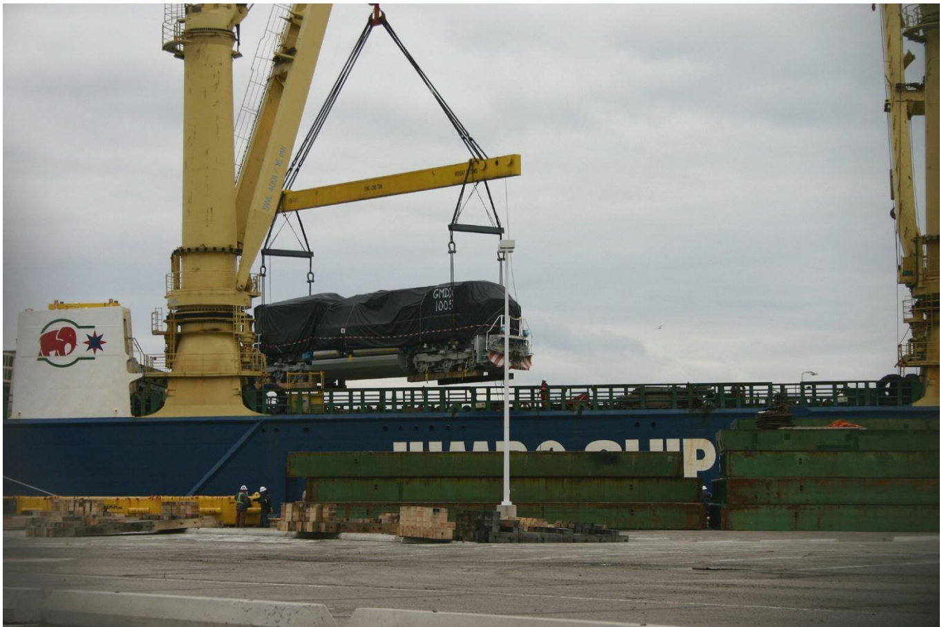
GMDX1005 swung onboard by MV Jumbo Vision heavy lift 600t ships crane then lowered into hold Photo Joe Zika
