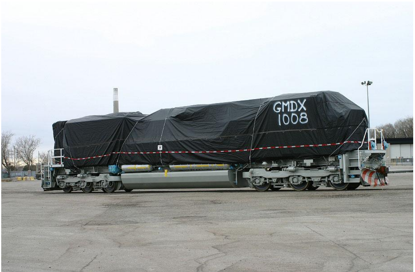
GMDX1008 on Toronto Harbour W52 November 19th 2008 showing locomotive on rails but covered in thick black plastic to protect the locomotive in transit on its long sea journey to Australia. GMDX is the EMD reporting marks that enables the locomotive to be hauled on US or Canadian Railroads. Photo by courtesy Joe Zika.
