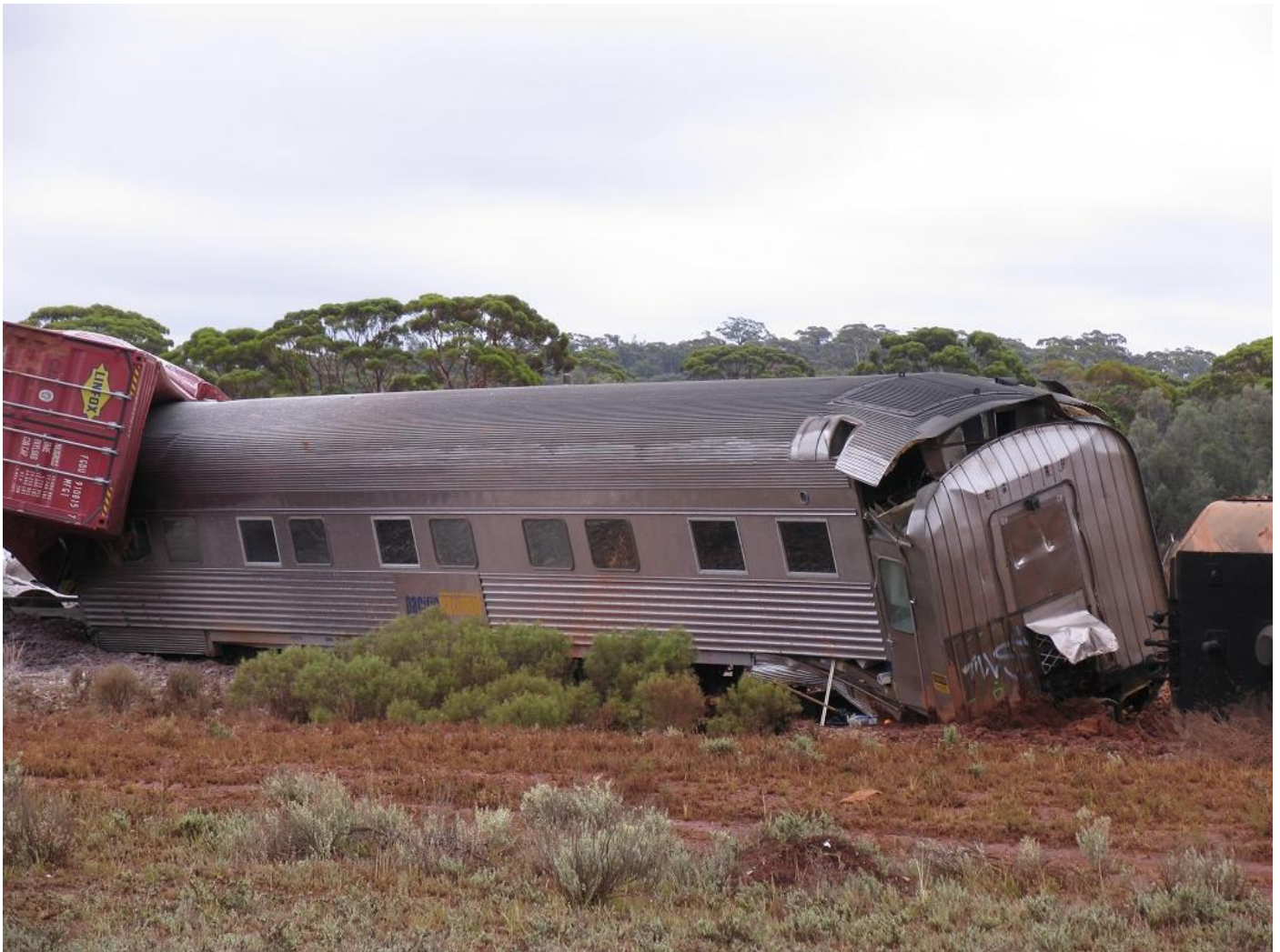
The crew car RAZY 289 though extensively damaged remained upright showing its strength of construction bending the empty container that landed on its roof in the 5PS6 derailment 30th January. Photo John Bollans
