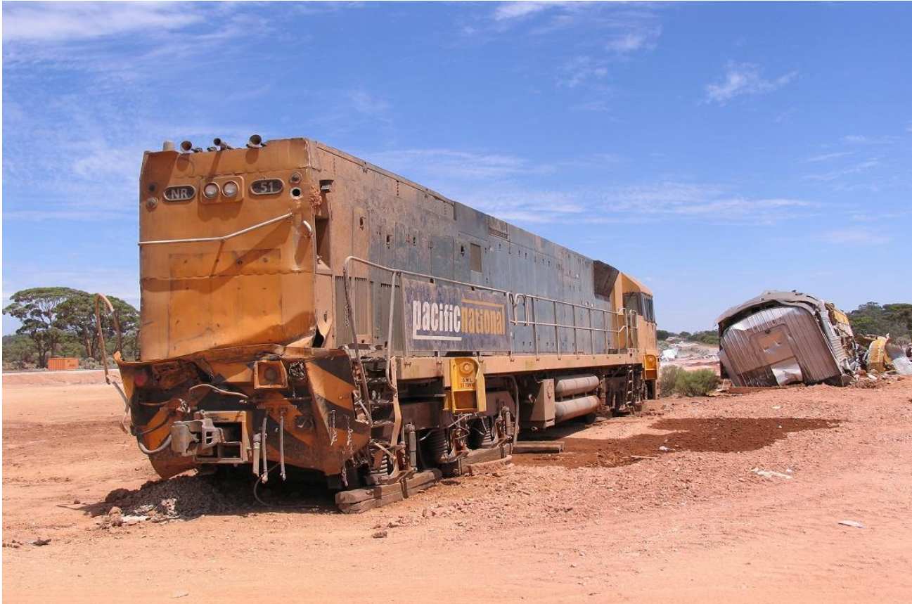
NR51 damaged in 5PS6 derailment now upright on February 15th and prepared to be lifted onto road transport to be hauled to United Group Rail Bassendean for assessment. Photo John Bollans
