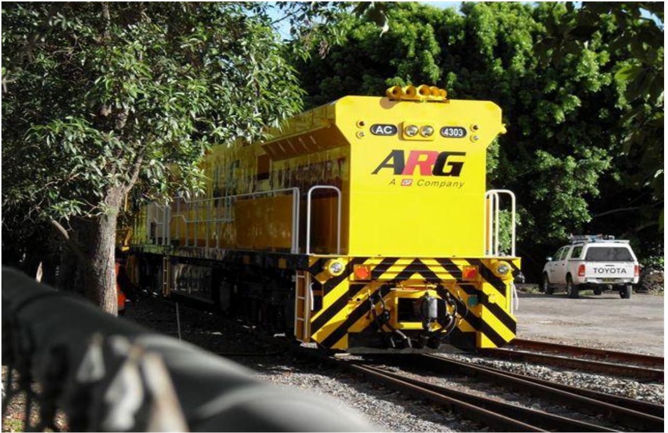
AC4303 being shunted from one part of Goninan Yard Broadmeadow plant to another on May 15th showing the large flared radiators on the long end hood. Photo Brad Coulter
