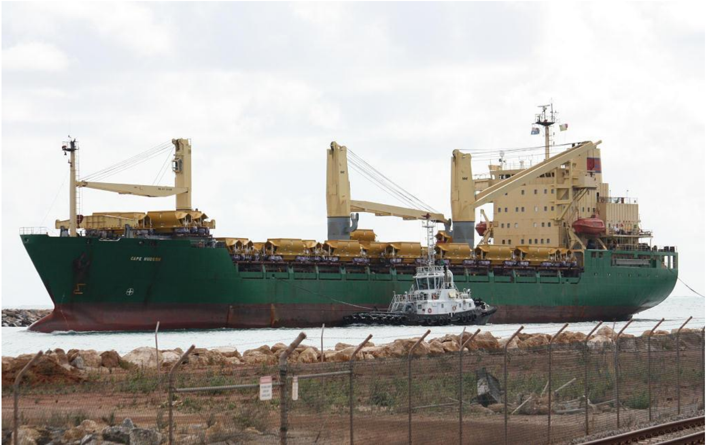
MV Cape Preston entering Geraldton harbour on May 23rd showing the deck covered in new ACHF ore cars being imported from China for use on Mt Gibson ore trains.
