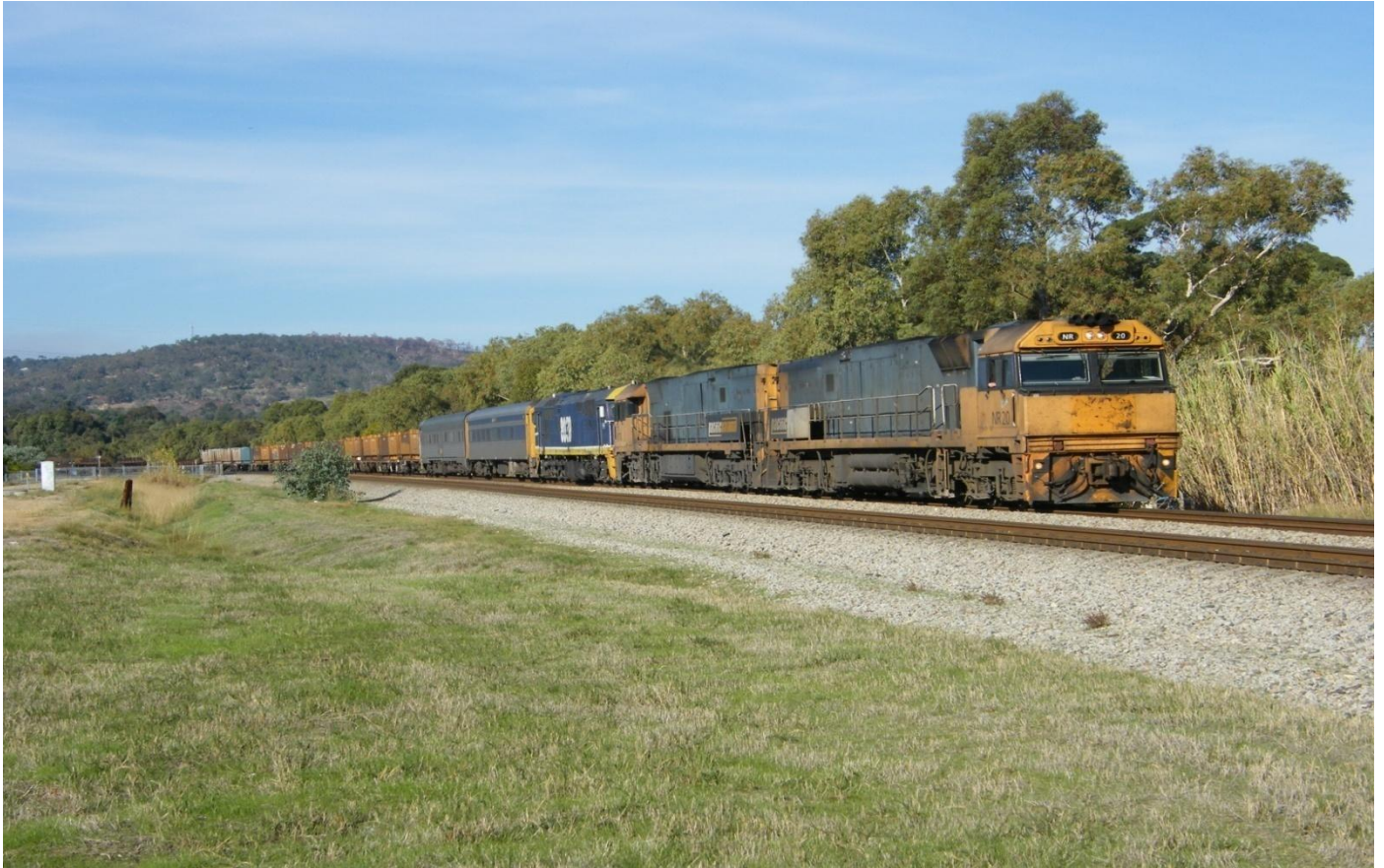
NR20, NR50 & dead attached 8039 Pacific National Kewdale yard shunter being returned following repair at EDI Port Augusta on 4WP2 steel train with two crew cars at Bellevue on June 7th. Photo Jim Bisdee
