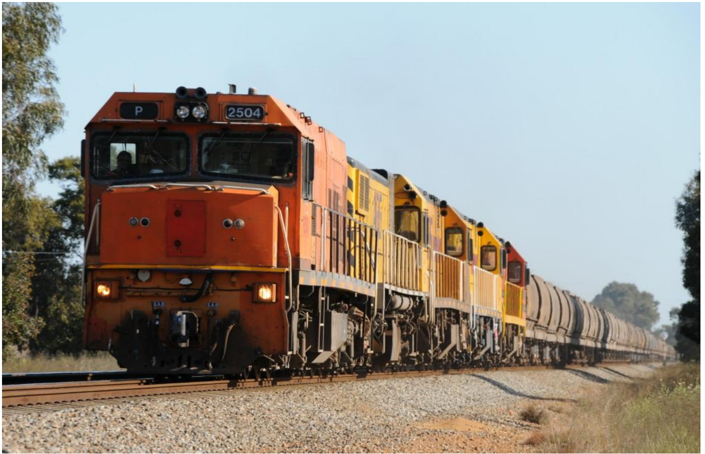
P2504 hauls dead DAZ1903, P2508, P2511 and P2506 on 7363 empty wheat train through Swan View on October 17th note the bowed frames on the P class locomotives. Photo Alex Mackay
