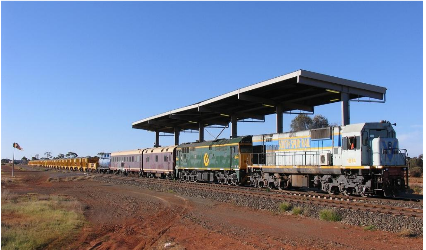
NA1874 & 8044 on 5MR1 South Spur Rail ballast train waiting to depart Parkeston on December 10th to undertake night ballasting between Coonana and Zanthus on ARTC Trans line. Photo John Bollans
