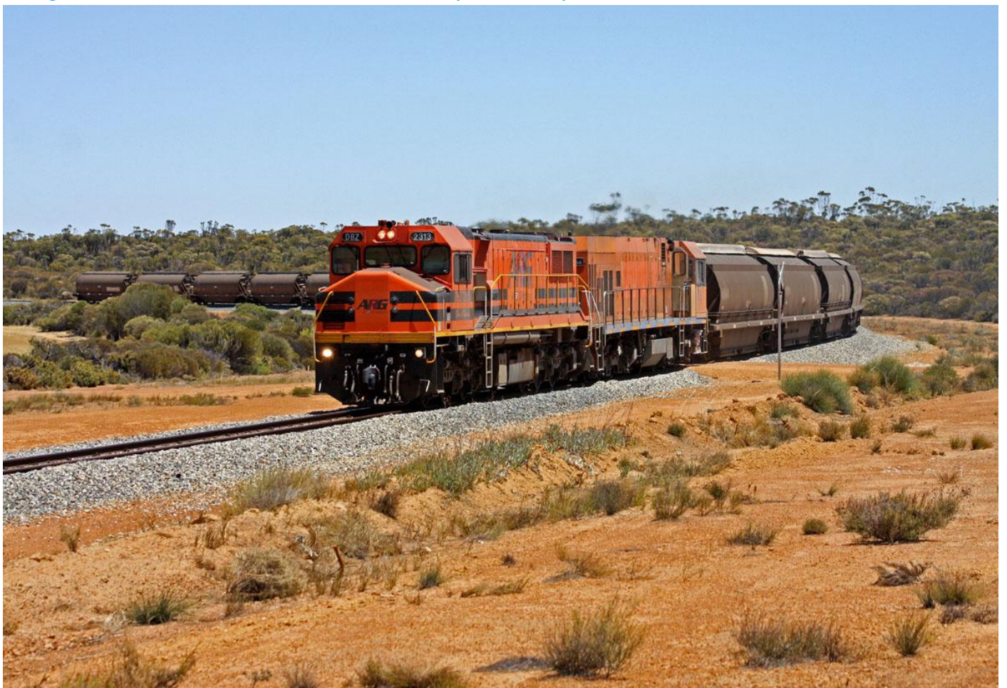
DBZ2313 & P2504 run 632 empty grain train on January 17th round the curves at Pederah on the Lake Grace to Hyden line that was laid with heavy rail and metal ballast in early 1980's. Photo Don Copley
