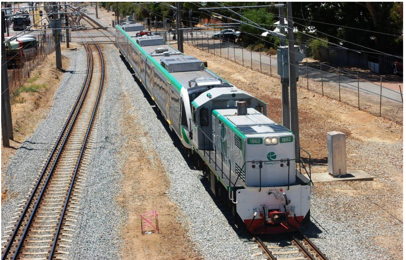
MA1862 runs 6UW2 empty railcar movement with EMU set #88 through East Guildford on January 22nd on the PTA dual gauge Midland line now laid with concrete sleepers. Photo Brendan Cherry
