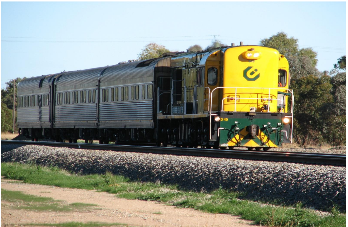
D49 runs AK car track recording train just east of Doodlakine on its return run from Avon Yard to Kalgoorlie on June 10th note video camera mounted above the coupler. Photo Stew Winston
