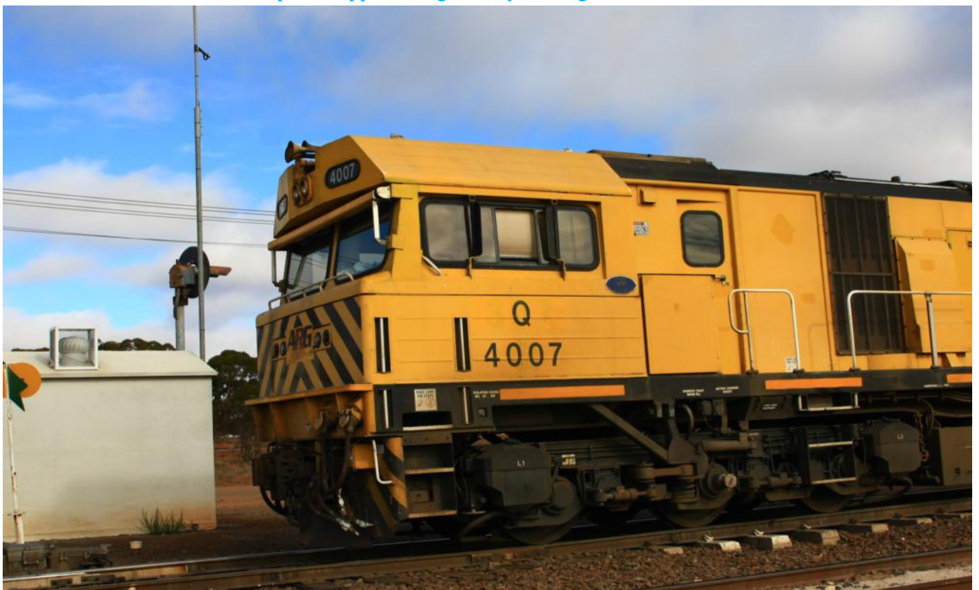
Q4007 at Parkeston on July 29th showing luxaflex blind over cab windows appears its for window protection when unit is a remote on DPU iron ore trains.
