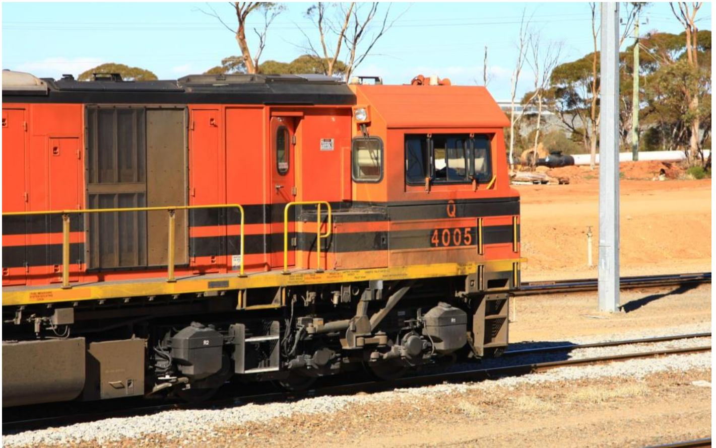
Q4005 at West Kalgoorlie on July 31st showing a light mounted on rear of cab as it appears its for easier crew changes in darkness by illuminating the steps and cab entrance.
