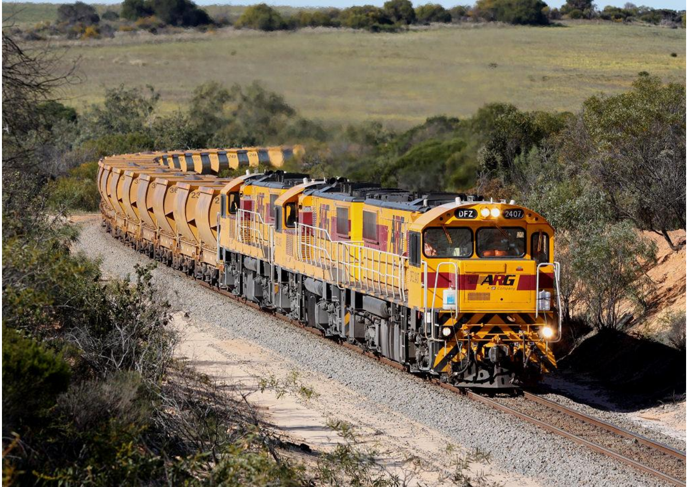
DFZ2407, DFZ2405 & DFZ2406 on 3715 90 wagon ore train trial at Wicherina on September 14th note the water containers and hoses on front of DFZ2407 to enable wet track testing. Photo Phil Melling
