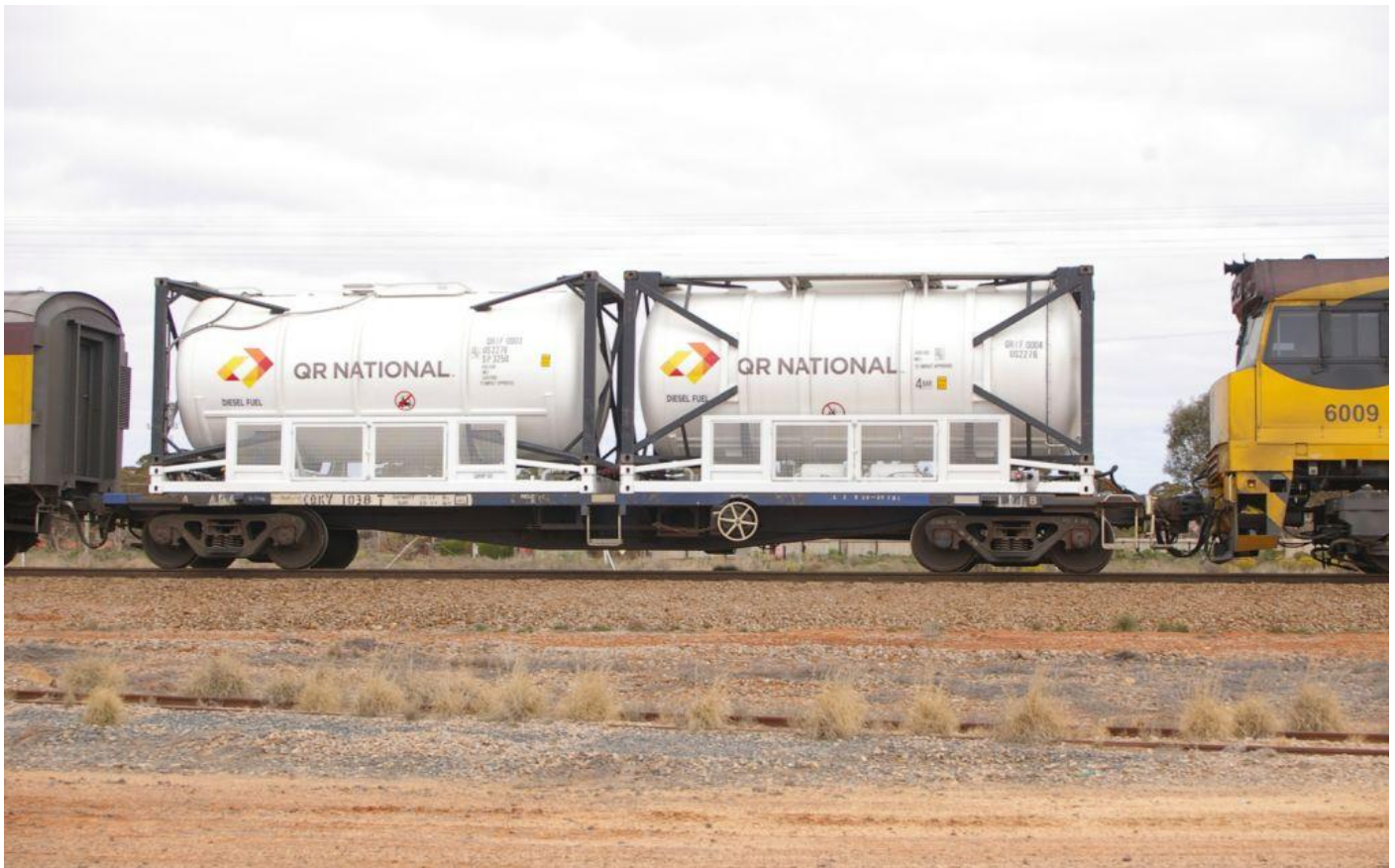
QR National inline refuelling tankers now in use on QRN transcontinental services fitted to CFCLA flattop behind 6009 & 6006 on 5MP1 at Parkeston on September 19th. Photo Peter Donaghy
