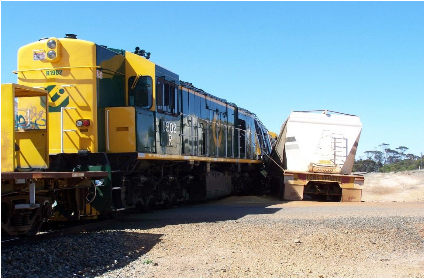
R1902 still on the track with RA212 derailed and leaning over at an angle of about 15 degrees with trailer against side of locomotive at Pootenup Road on 12th. Photo Daryle Phillips
