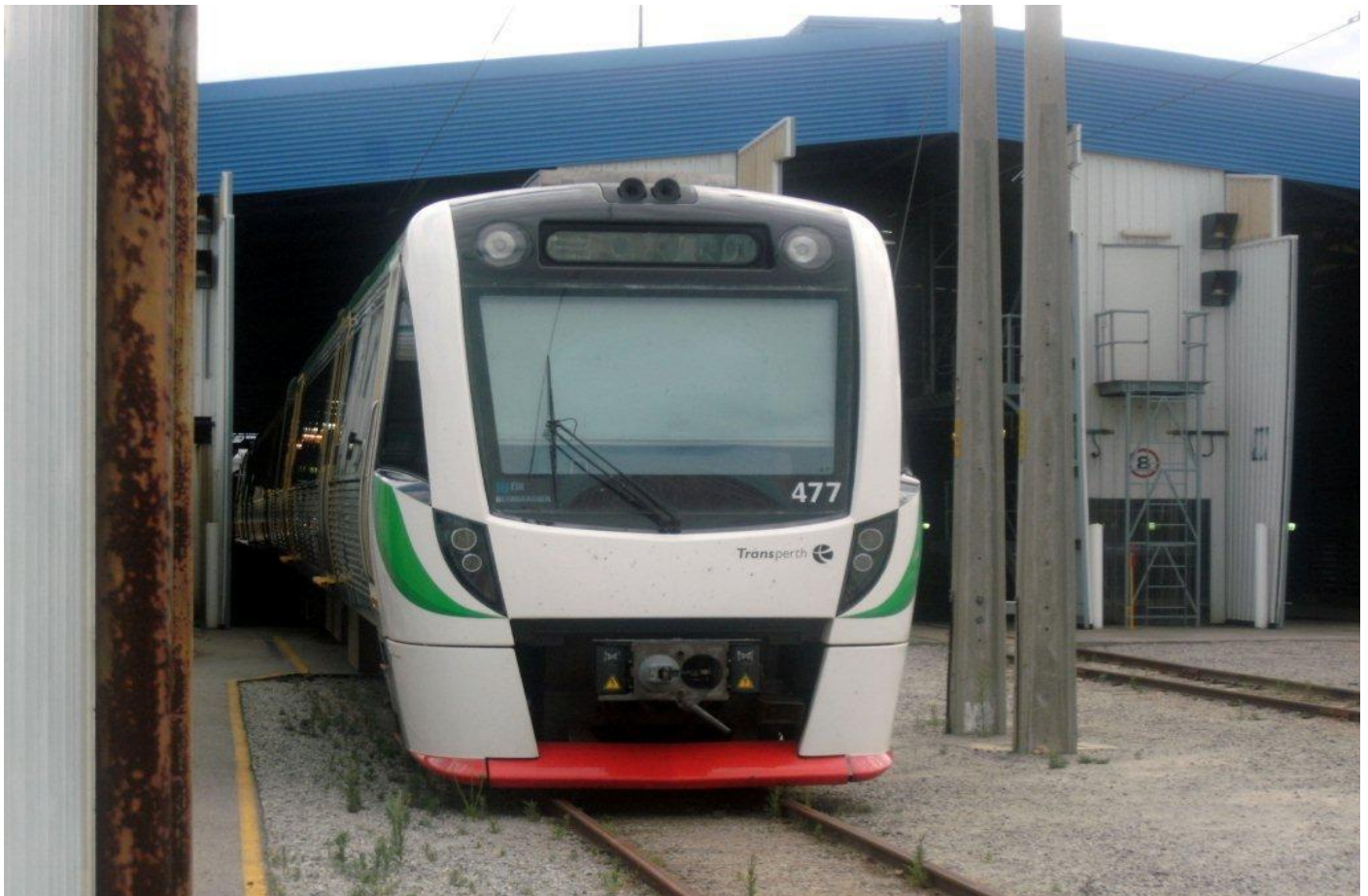
EMU B series set #77 at Claisebrook depot December 22nd cameras installed on roof to monitor catenary.
