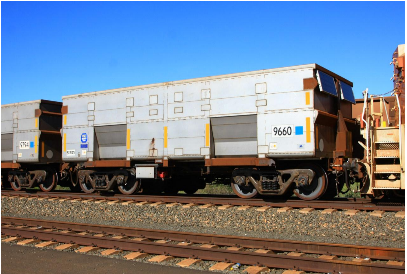
9960 an instrumented car at Bing on February 8th note solar panels and batteries. Photo Toad Montgomery
