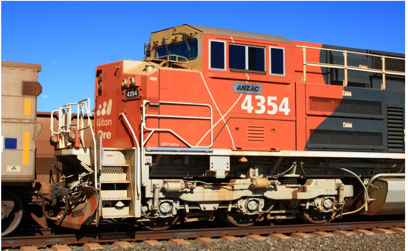
4354 at Bing on February 8th showing modifications made to handrails.
