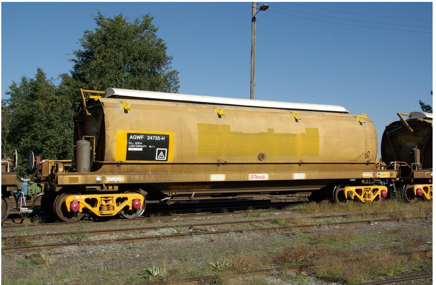
AGWF24735-H former narrow gauge XW grain wagon converted to standard gauge for use hauling export grain to Port Kembla at Goulburn shortly after arrival on April 3rd.
