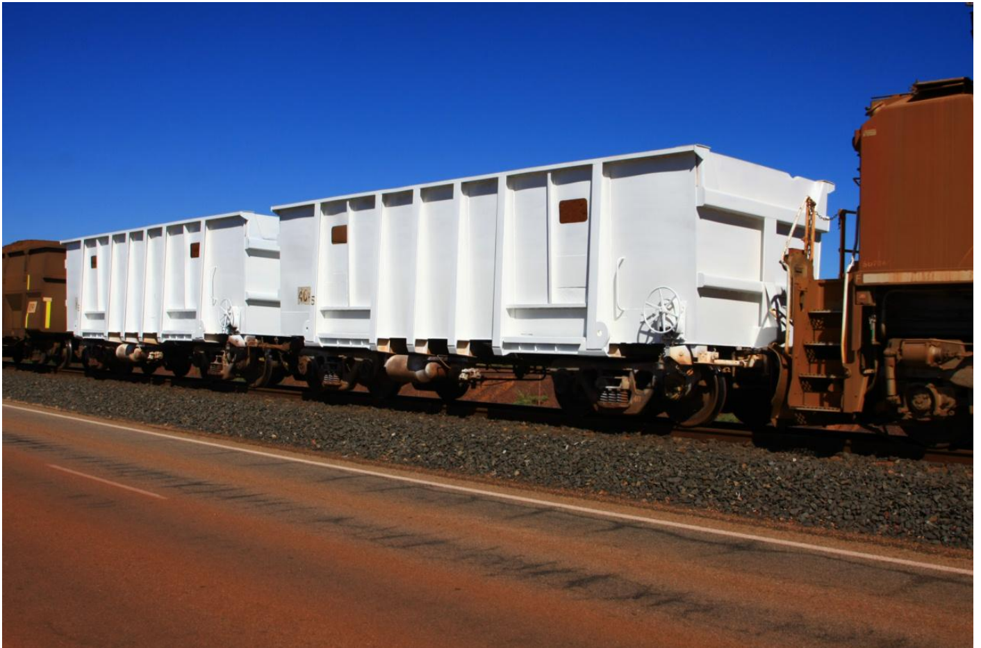
New style index cars April 14th are used at Finucane Island on CD4 car dumper. Photo Toad Montgomery
