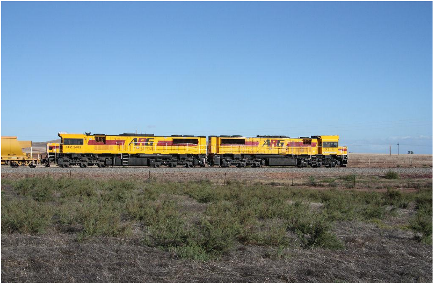
DFZ2405 and DFZ2404 showing difference between the original lower Queensland cab and modified larger rebuilt WA cab on April 26th at Moonyoonooka. Photo Phil Melling
