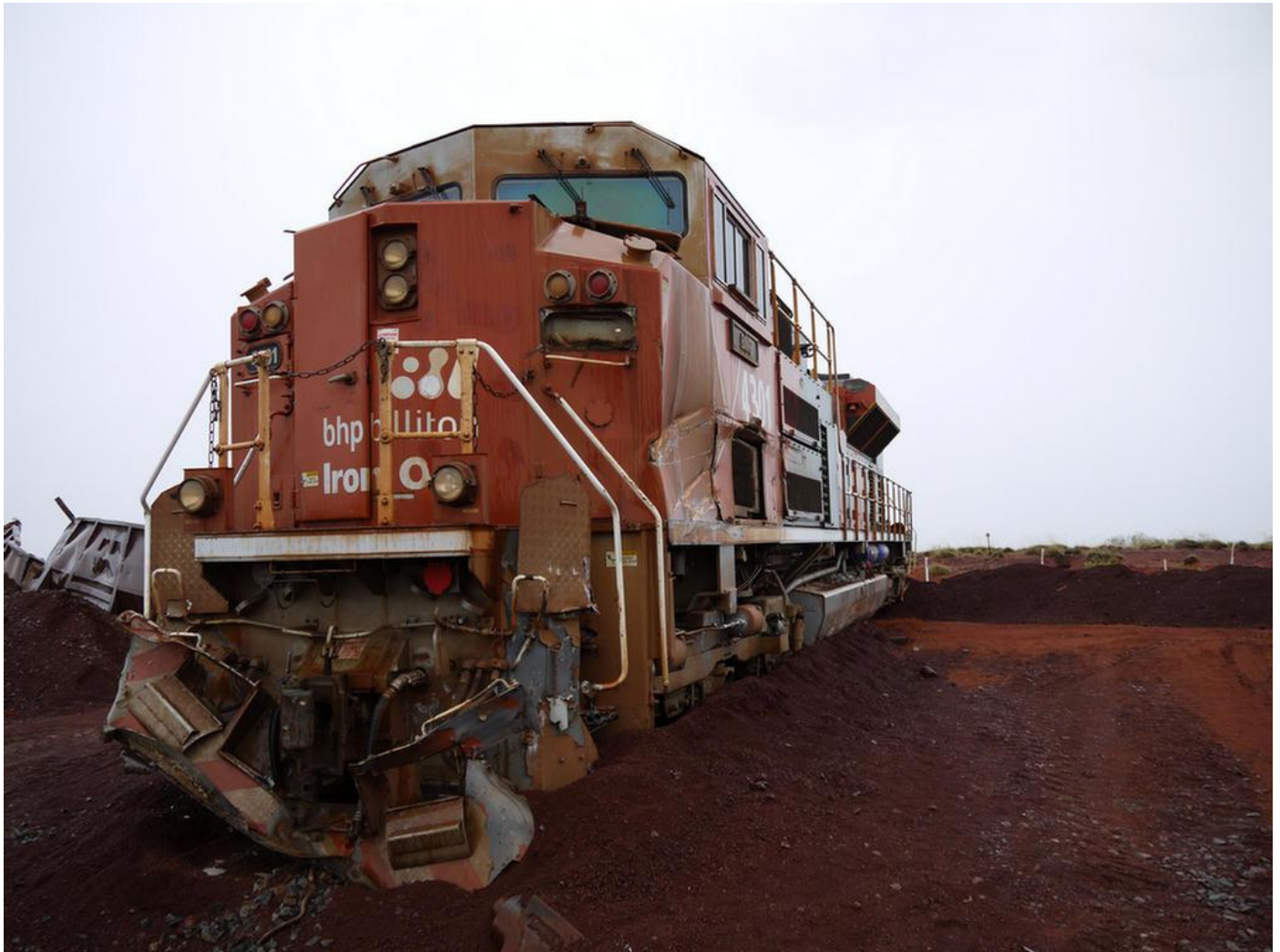
Derailed damaged SD70ACE 4301 being prepared to be recovered on June 6th. Photo Richard Searle
