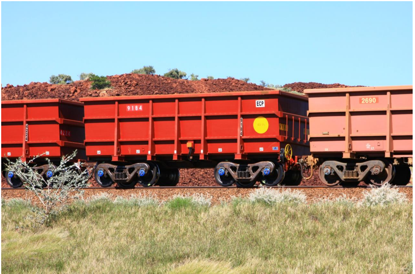
Older style Bradken ore cars fitted for ECP braking at Dugite loop on June 2nd.
