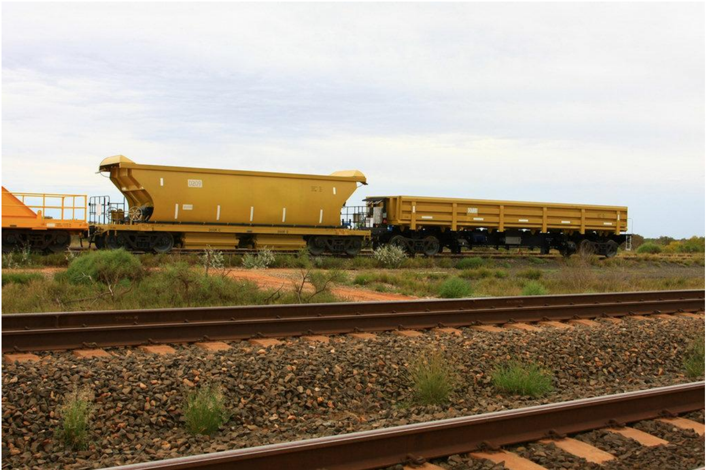
New ballast hopper with a side dump car at BHOBIO Bing Yard on June 6th. Photo Toad Montgomery
