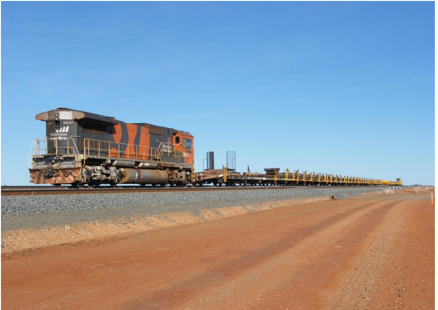
5637 on rail train recovering old rail on Mt Newman main at Mooka on June 19th 2011. Photo Jim Bisdee
