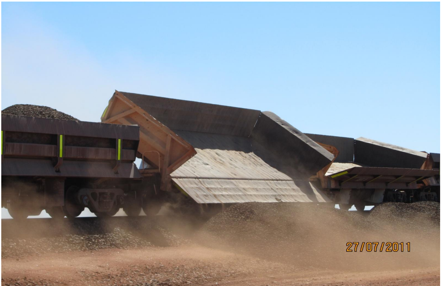
BHPBIO side dump cars dumping at new Asset Protection Super Site at 27.8km on Mt Newman main.
