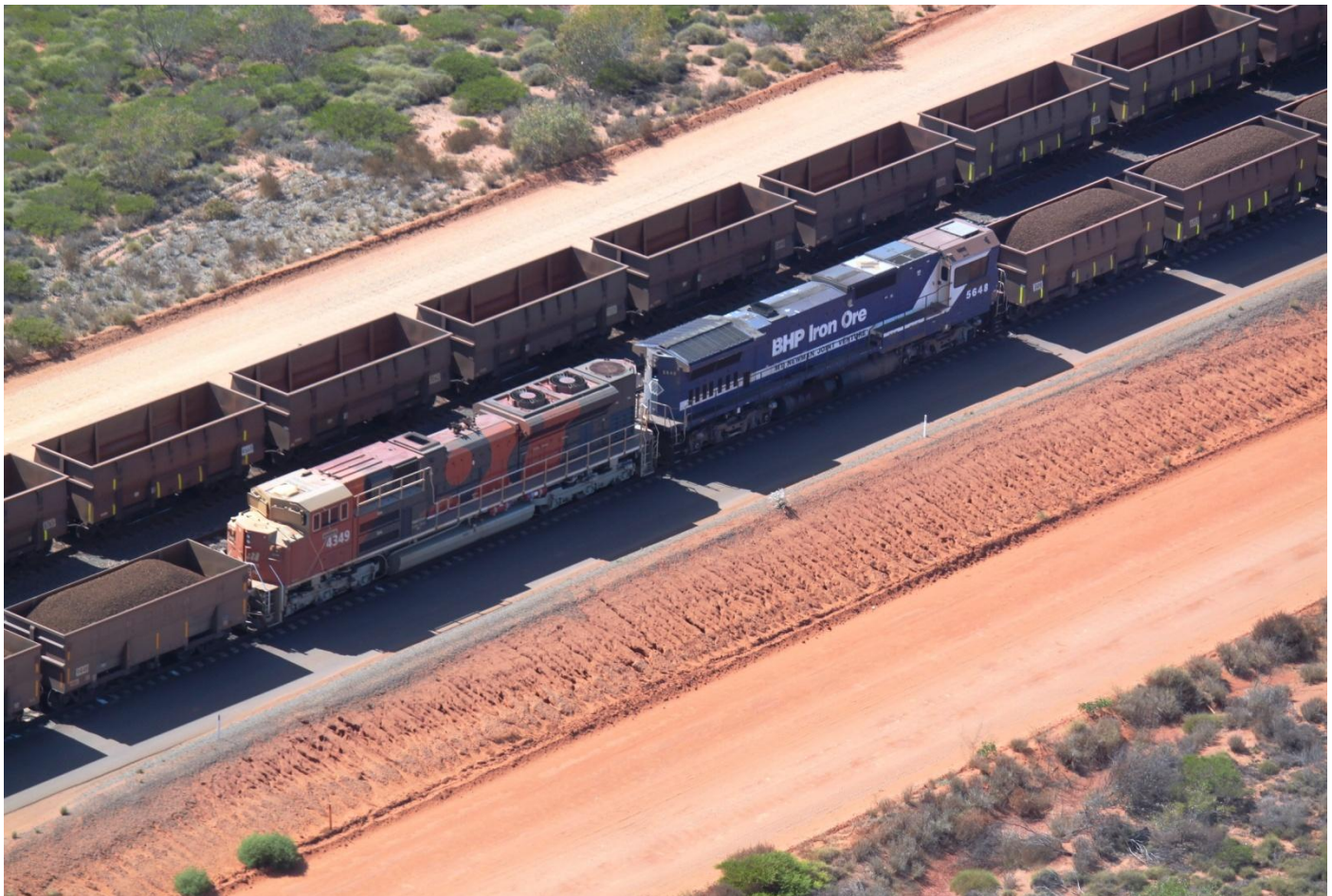
4349 & 5648 mid train DPU units on loaded ore train passing empty at Bing October 15th. Photo Baden Tidd
