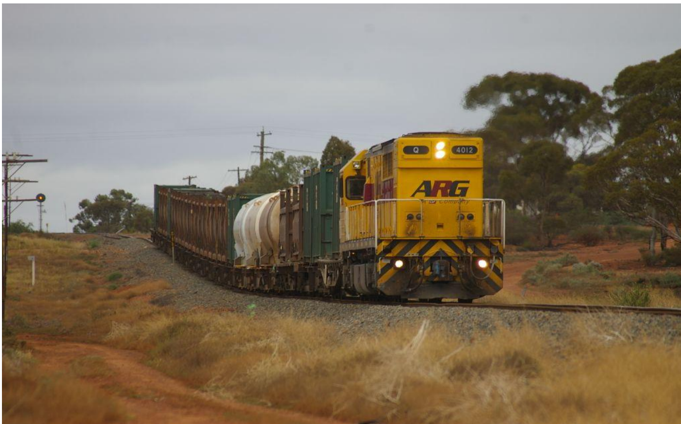
Q4012 on 6029 sulphur train on October 29th just north of Kalgoorlie on line to Leonora, this line built over a century ago to narrow gauge converted in 1974 but retaining its minimal earthworks. Photo Peter Donaghy
