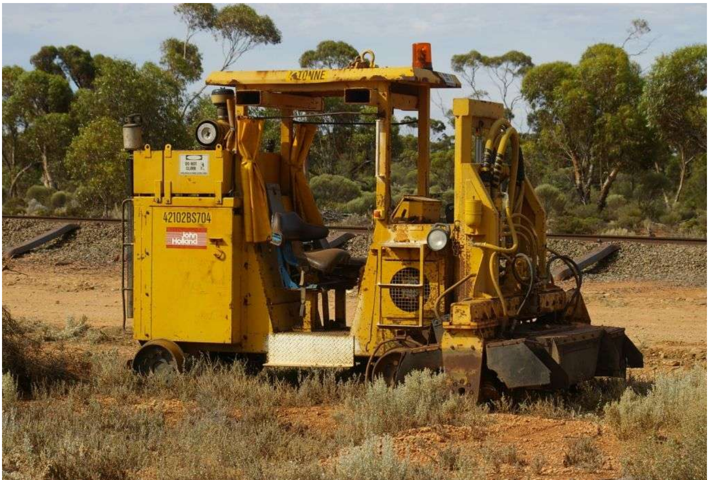
Sleeper replacement machine at Binduli February 12th note steel sleepers to be inserted adjacent to track.
