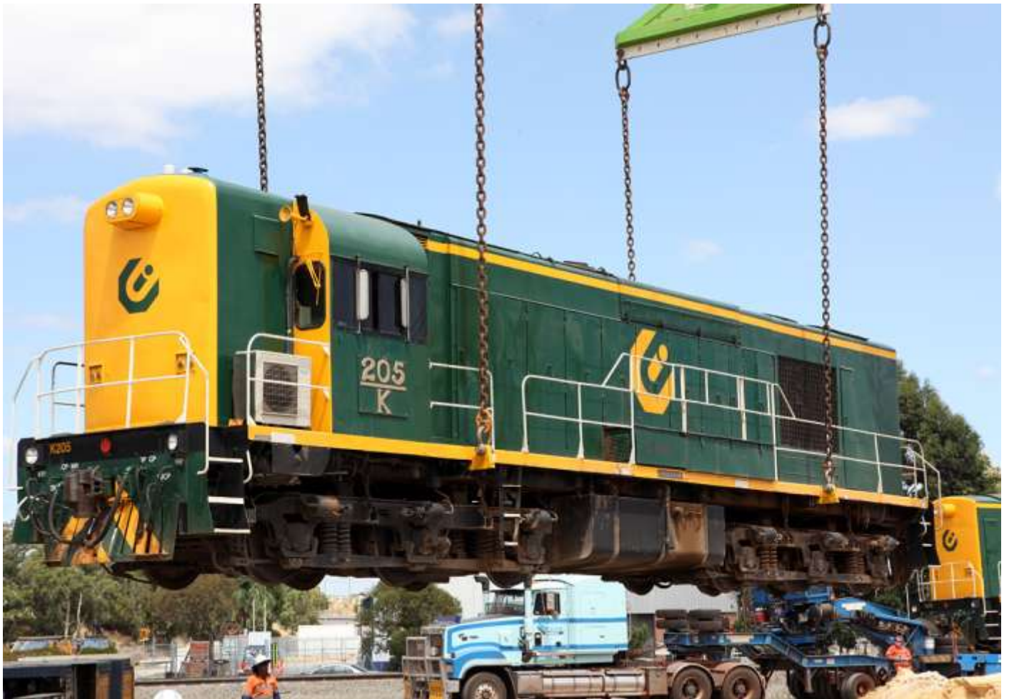
K205 lifted of road transport then being put on rail at Bellevue February 25th.
