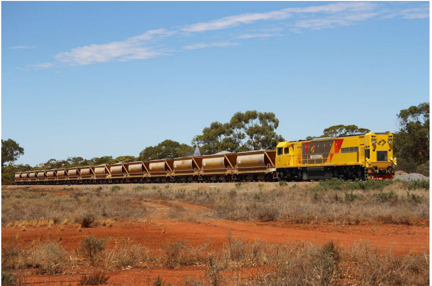
ACN4147 pushes CFCLA CHOY ballast wagons [previously on standard gauge working on BHPBIO expansion] through water spray to limit dust at Gutha March 5th. Photo Phil Melling
