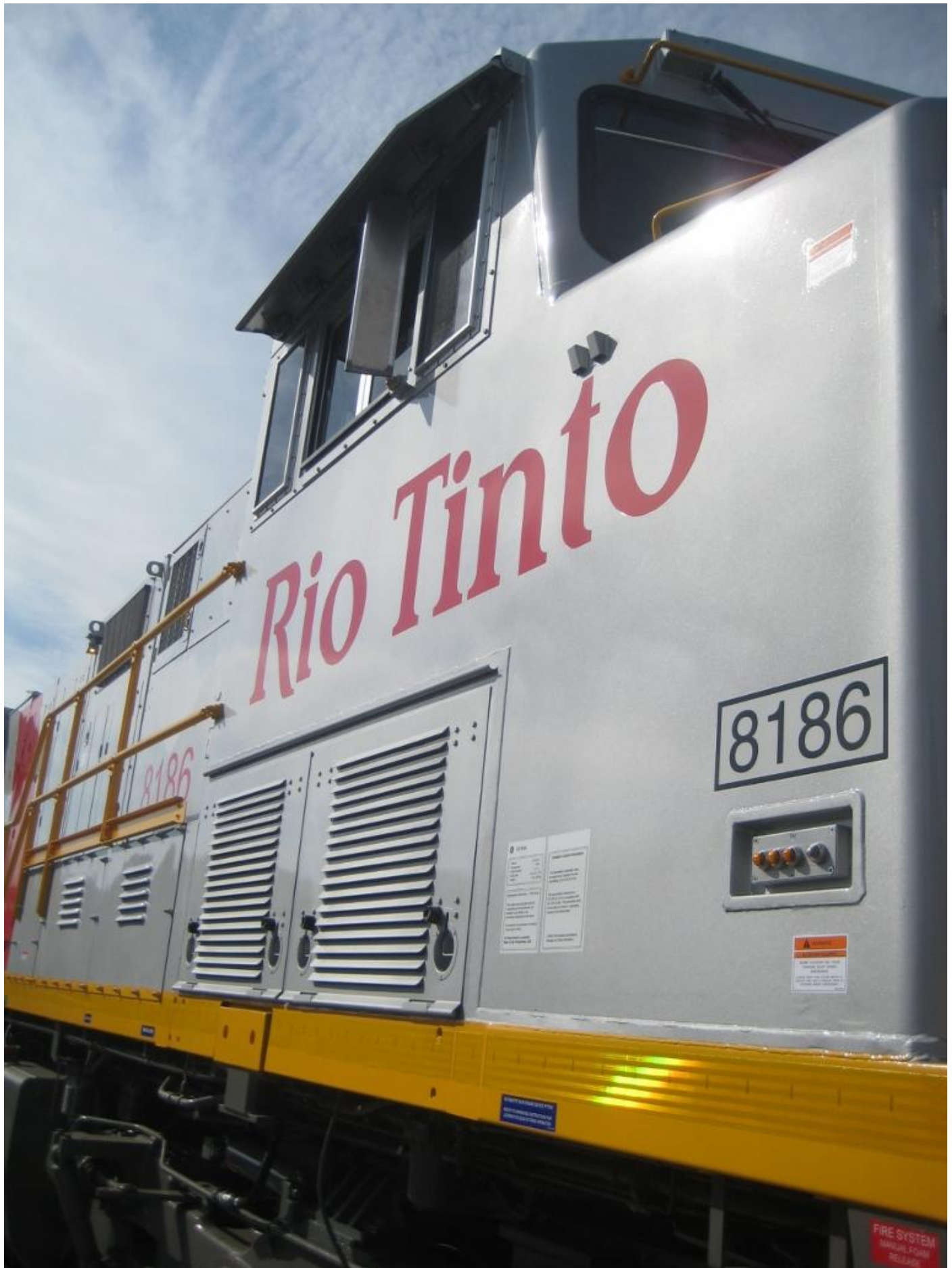
Cab profile of Rio Tinto ES44DCi locomotive 8186 final the locomotive of this contract in General Electric yard Erie Pa undergoing acceptance testing March 11th. Photo Ian White END 12 of 12
