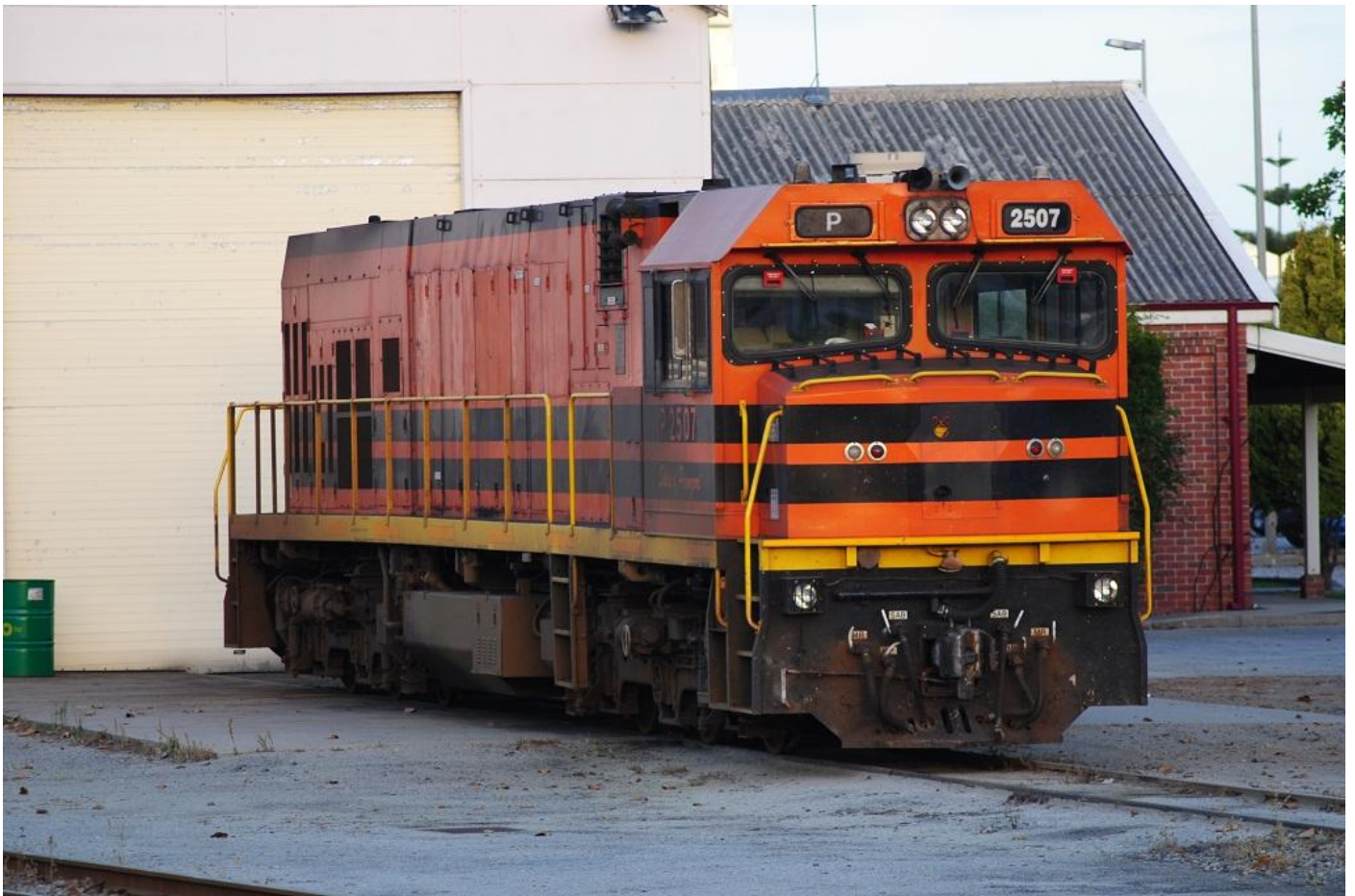
P2507 at Albany loco May 23rd showing quick release windscreen and ladder on nose.
