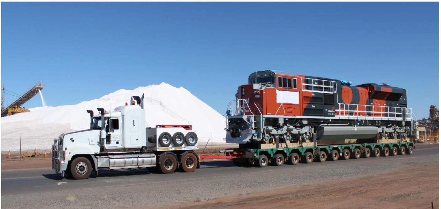
SD70ACe on transport float being hauled from Port Hedland Town wharf to hardstand at Nelson Point to be placed on rails to allow commissioning May 26th. Photo Baden Tidd
