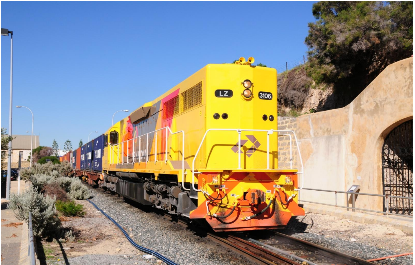
LZ3106 on 6142 container train at Roundhouse Fremantle with water being sprayed on the track as a noise reduction agent to reduce flange squeal on the sharp curve May 18th. Photo Graham Edwards
