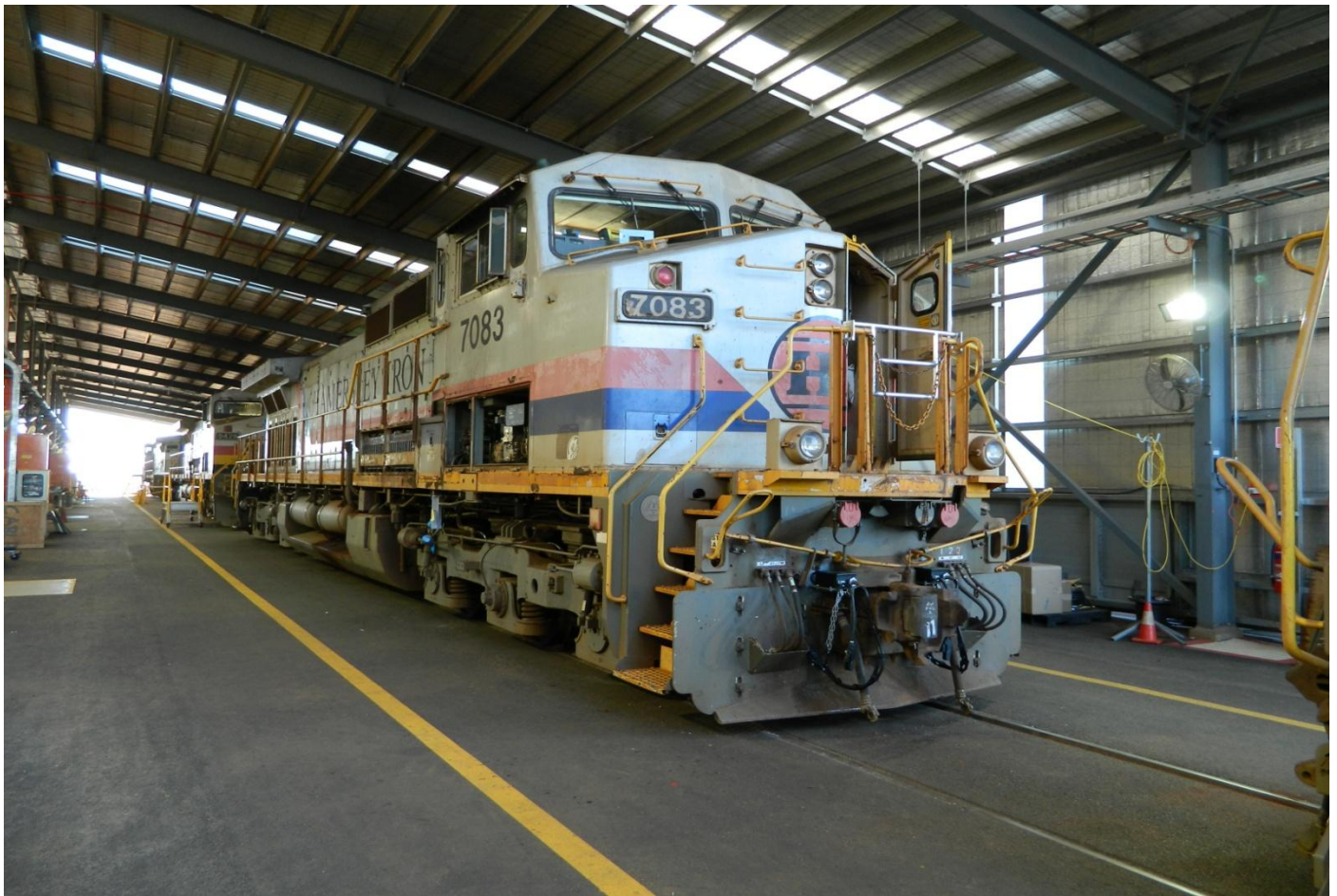
7083 in 8 Mile workshop showing ECP being braking fitted July 18th.
