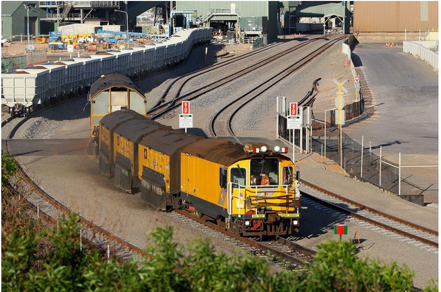
MMY32 QRN rail grinder grinding lines at the Geraldton Port September 15th.
