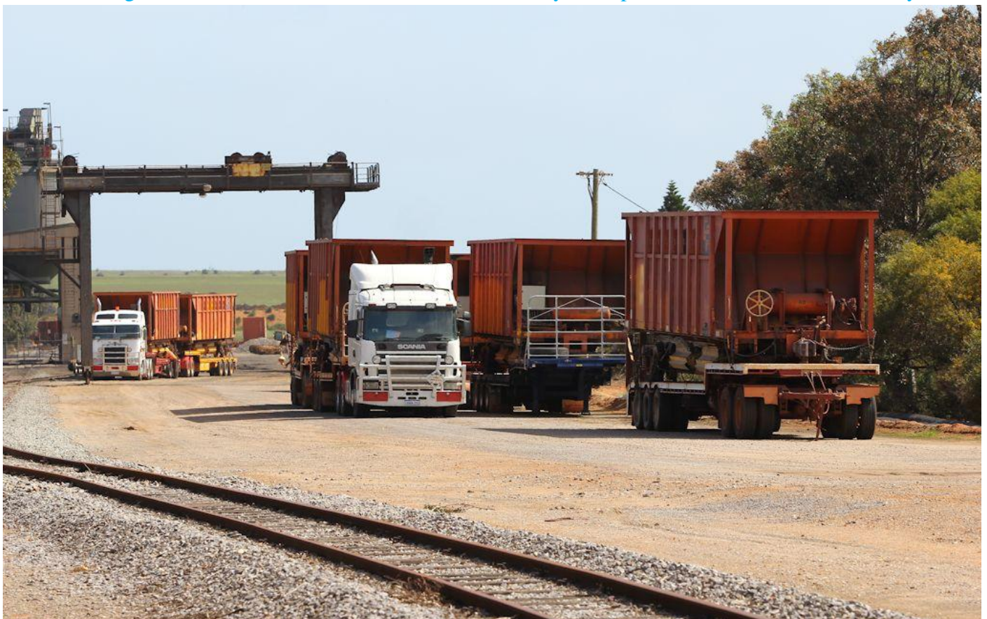
Some CFCLA CHAY 2xpack hoppers were converted into ballast wagons for use on Mid West upgrading here loaded on semi trailers ready to be hauled out at Narngulu at their end of use 4/9. Photo Phil Melling
