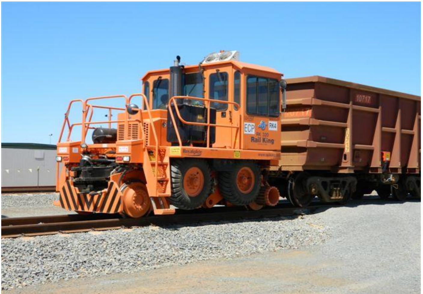
RK4 Rail King hauls EPC brake converted ore cars at 8 Mile yard September 5th.
