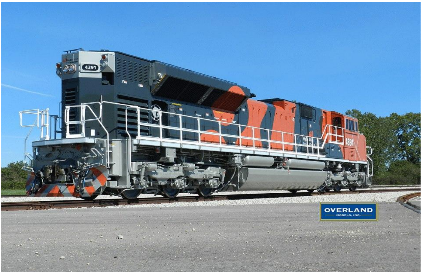
#4391 showing gattings protection on B end at EMD Muncie 11/9. Photo Overland Models Inc Brian Marsh
