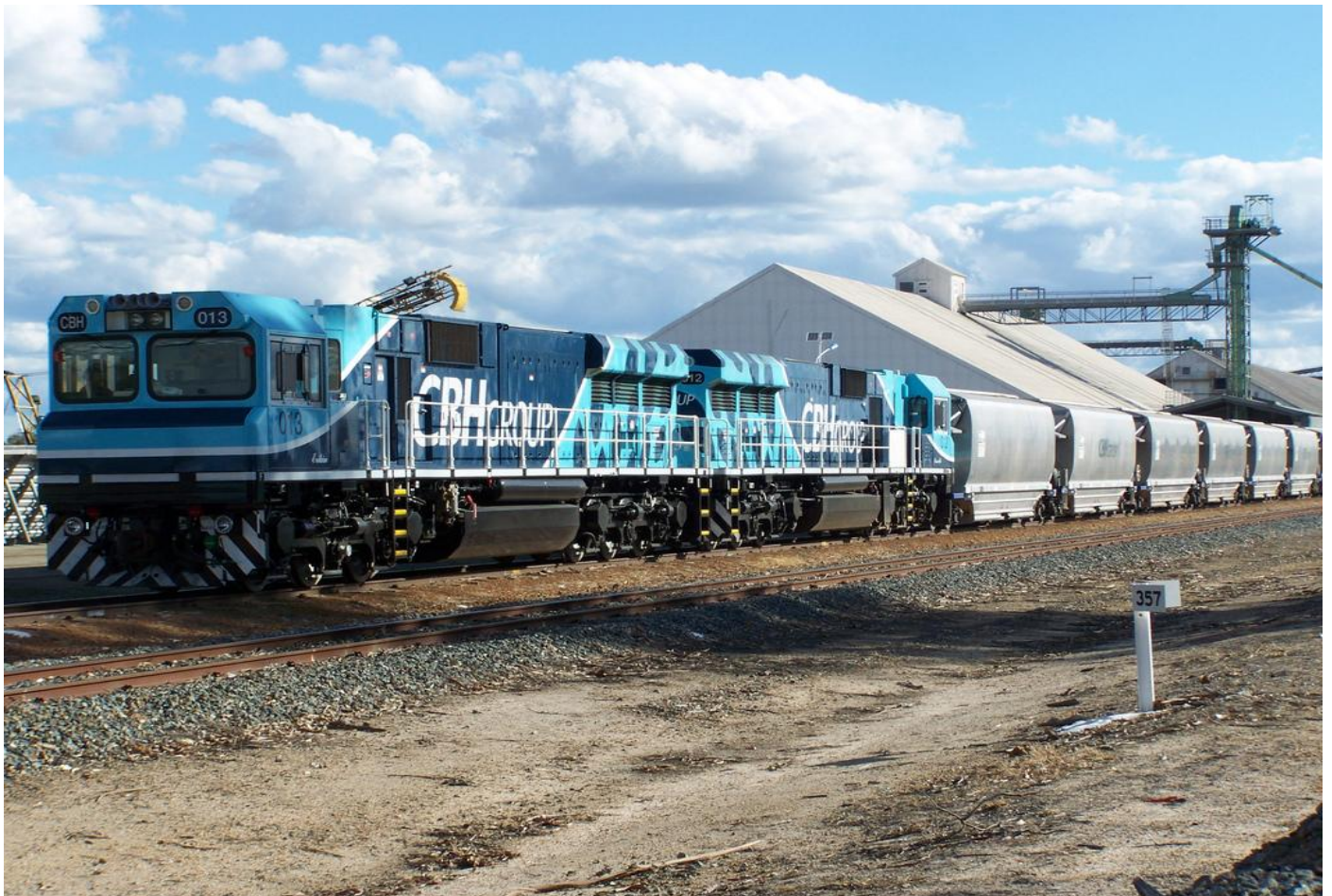
CBH013 & CBH012 were first of the heavier and more powerful MP33CN locomotives to enter service.
