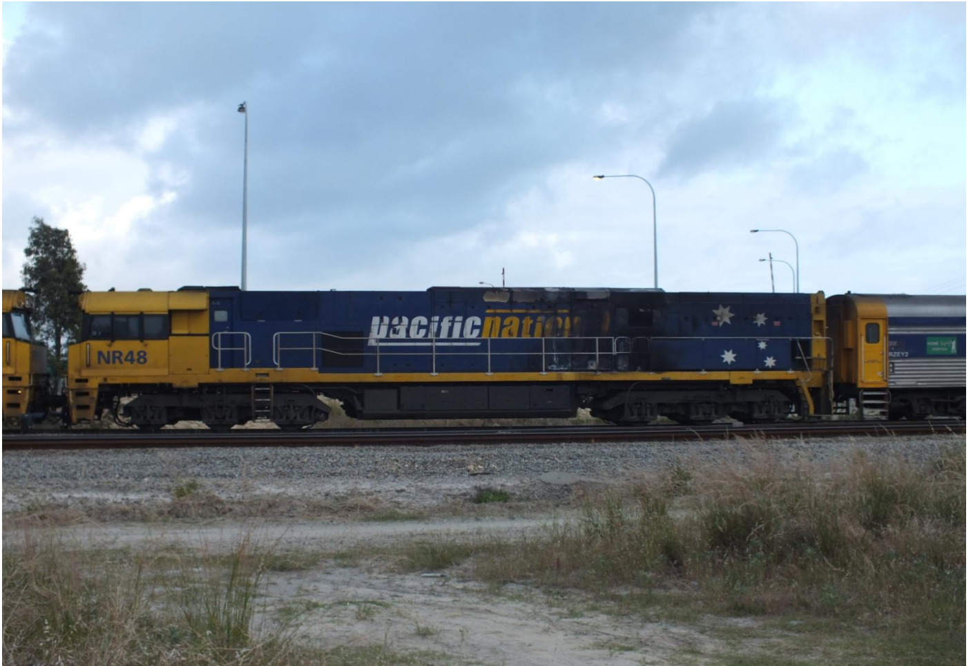
NR48 showing its fire damage entering Pacific National Kewdale on 4MP5 October 13th. Photo Jim Bisdee
