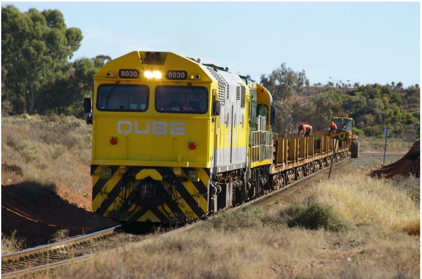
Q8030 & K206 propells loaded rail train to end of Brookfield territory at Kalgoorlie to drop new heavy rail as part of re-railing of EGR from Koolyanobbing to Kalgoorlie October 28th. Photo Peter Donaghy
