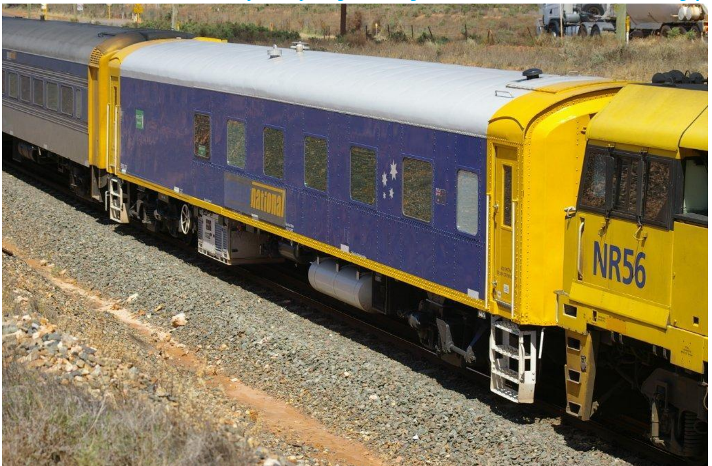
BRS225 rebuilt following shunting accident at Port Augusta at West Kalgoorlie December 1st note there are now no rivets on this former Spirit of Progress car the in repaired area. Photo Peter Donaghy
