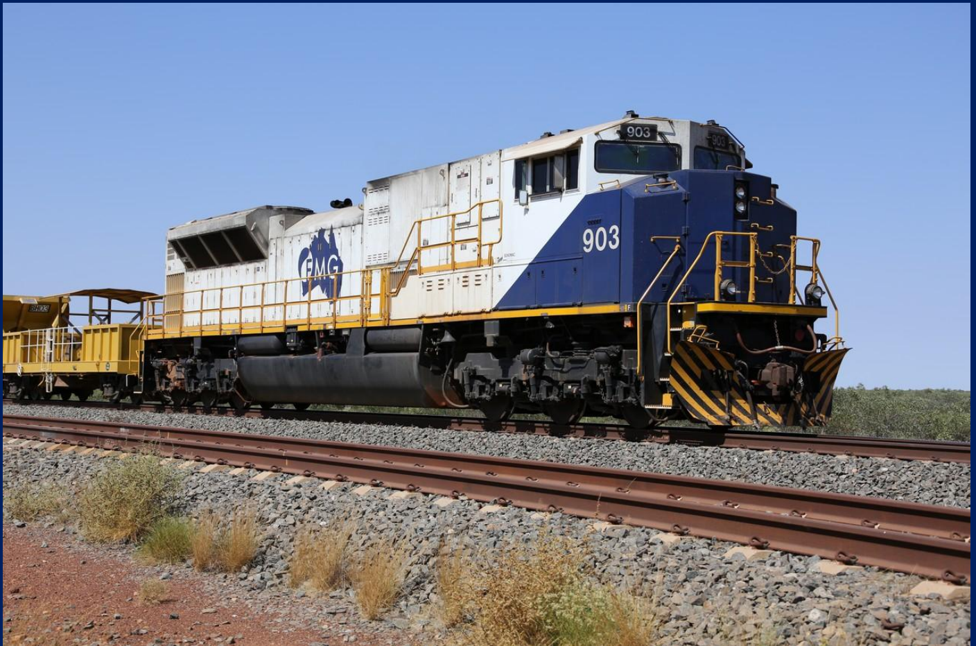
FMG SD90MAC-H 903 with BP2 ballast plough on ballast rake Barker Siding 17/9. Photo Toad Montgomery
