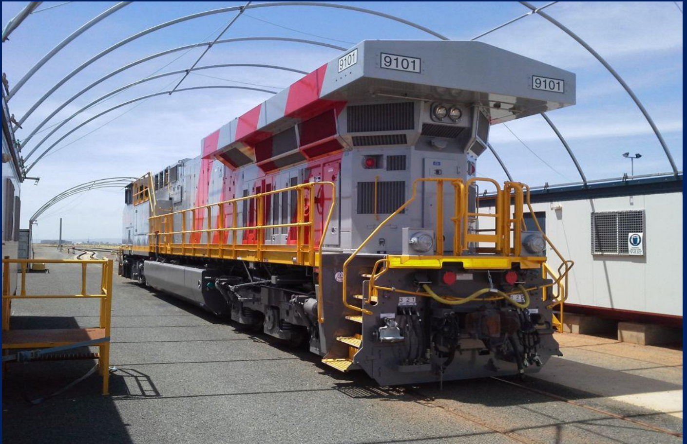
ES44ACi 9101 undergoing commissioning at 8 Mile 12/02, note massive radiators.
