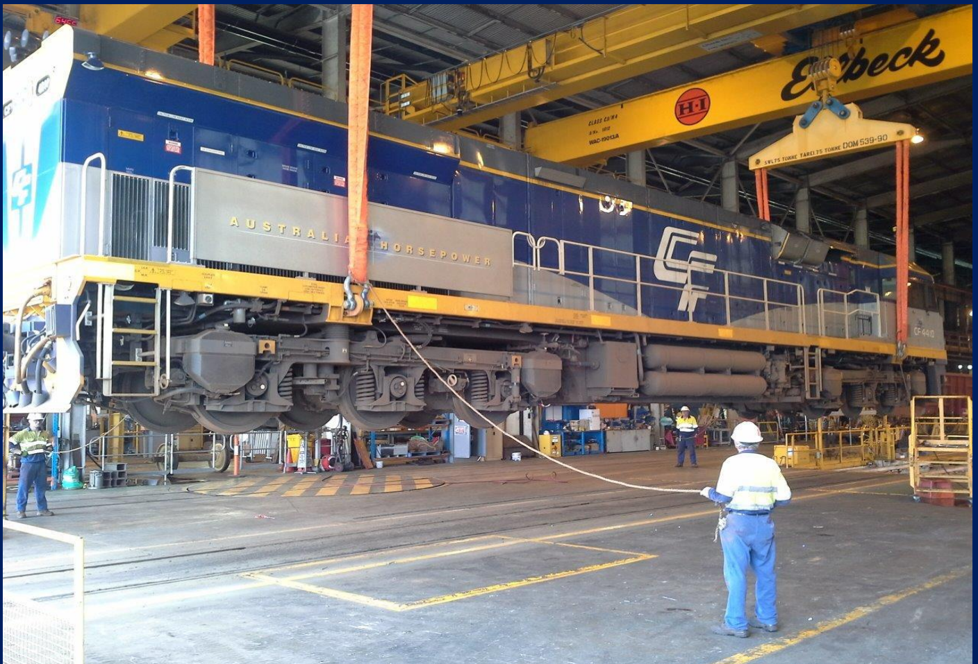
CF4410 being lowered onto rail in 7 Mile workshop Dampier May 7th.
