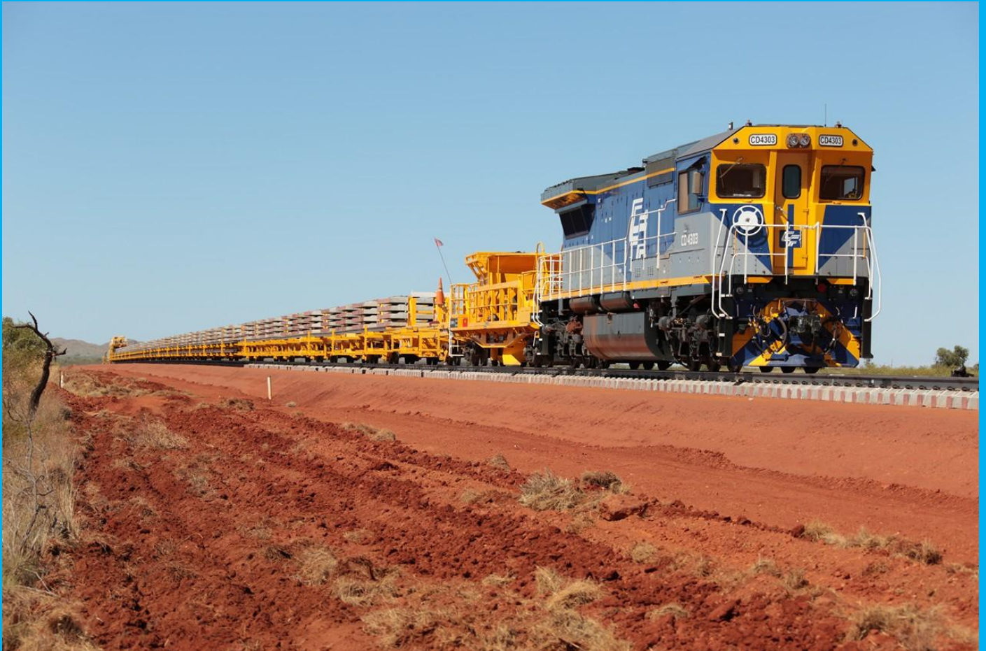
CD4303 on Roy Hill sleeper train with tracklayer on rear [that is leading when laying track with locomotive pushing] about 90km south of Port Hedland 6th August.
