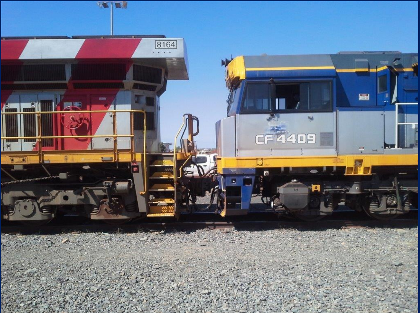
GE ES44DCi 8164 multi coupled to GE/UGL C44ACi CF4409 during coupling up testing at 7 Mile workshops Dampier August 28th to ensure CFs can be trailed behind EVOs and Dash9s. Photo Gary Lamb
