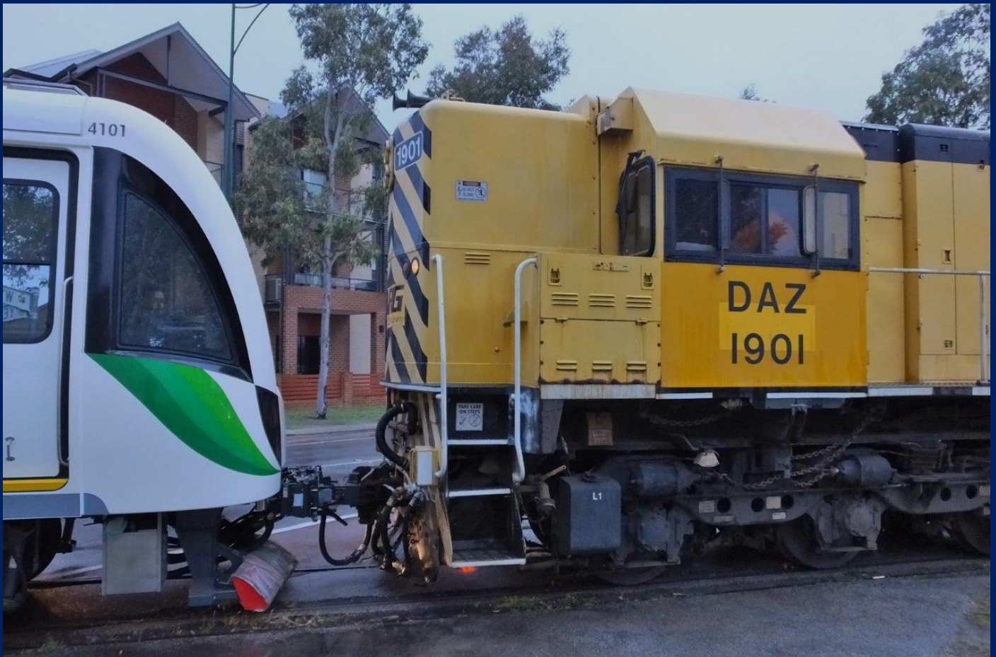
DAZ1901 hauling B series set #101 showing coupling transition piece Midland 29/8.
