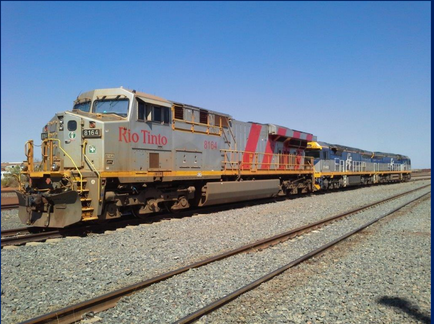
EVO 8164 with C44ACi CF4409 & CF4410 during coupling tests at Rio Tinto 7 Mile workshop Dampier on August 28th note the hight difference between US and Australian domestic locomotives. Photo Gary Lamb
