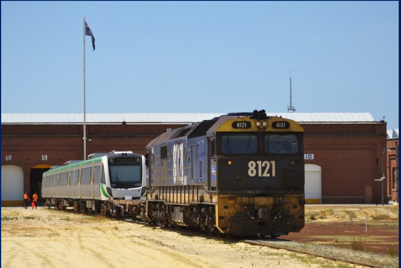
8121 on 3P31 propelling EMU set 103 into 6 road old workshops for fitting of its powered bogies 4/11.
