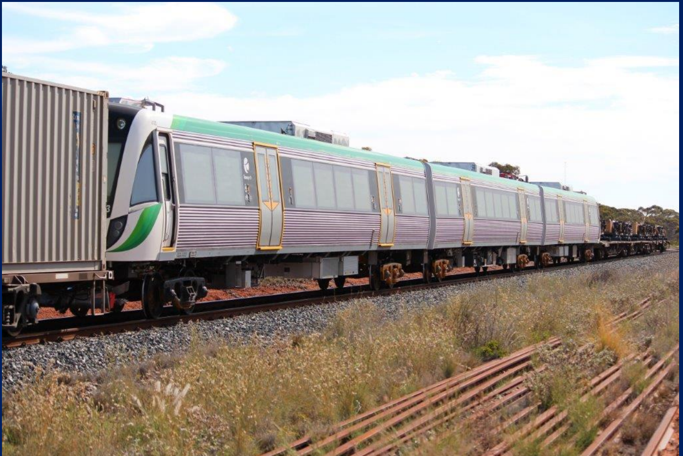
New PTA EMU set #103 on s/g transfer bogies at rear 5MP2 steel Binduli 2/11. Photo Peter Donaghy
