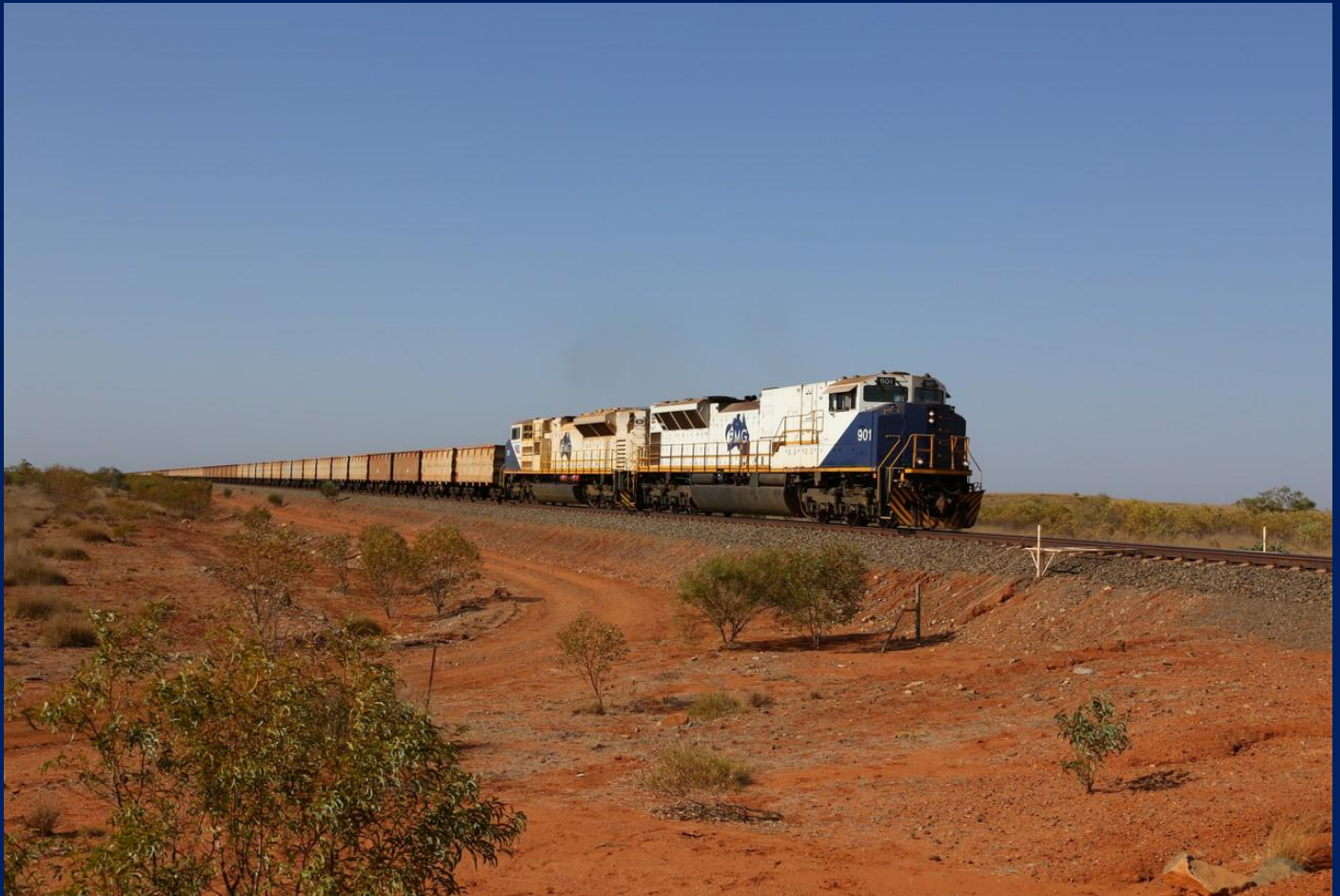
SD90MAC 901 [locally re-motored with 16-710 engine] & SD70ACe 701 on empty ore at 36km 26/11.
