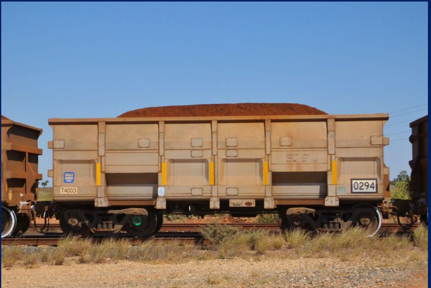
BHPBIO ore car showing has ECPB brakes and capacity 138.4t tare 21.6t Boodarie 12/7. Photo Jim Bisdee
