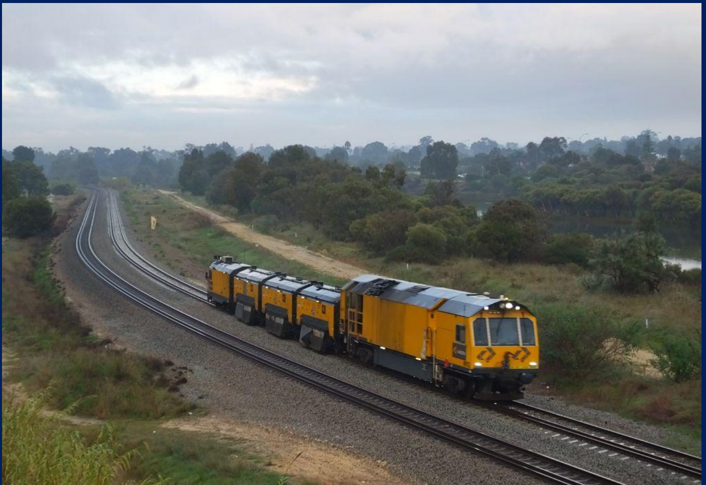
MMY32 Aurizon rail grinder in the rain running thru Wattle Grove July 4th.
