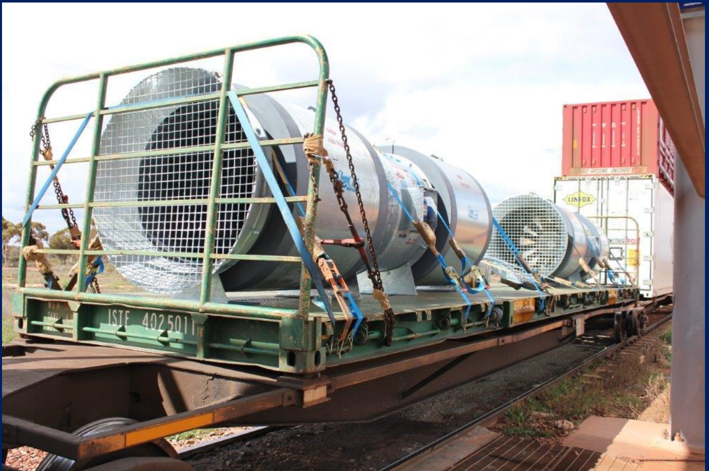
Big ventilation fans used in underground mines on skeleton wagon Parkeston 22/8. Photo Peter Donaghy
