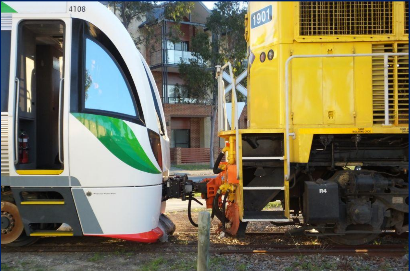
DAZ1901 transition coupler attached new EMU car 4108 at Midland August 14th.
