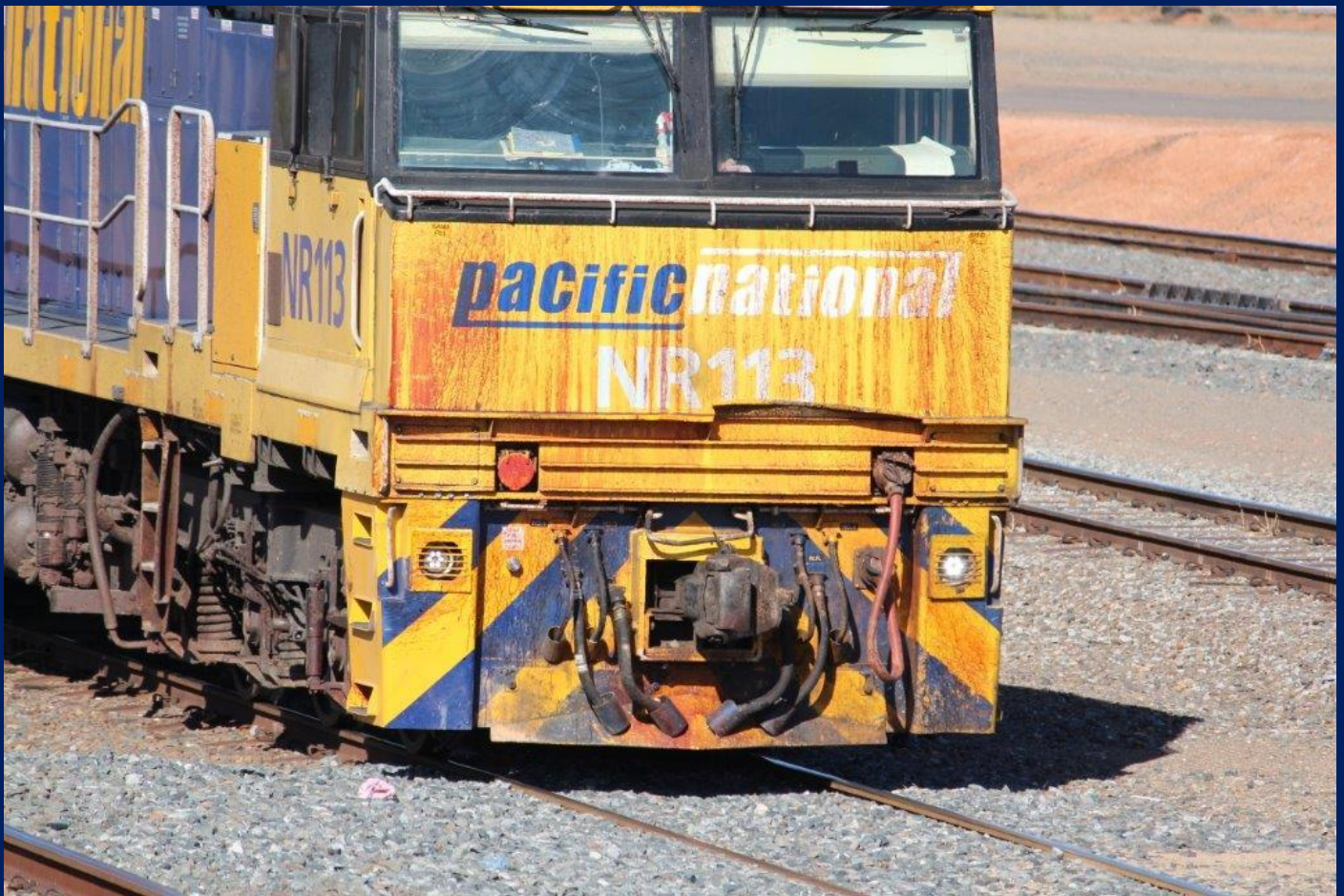
Close up of damage to NR113 after hitting a camel in desert east of Kalgoorlie 1/12. Photo Peter Donaghy
