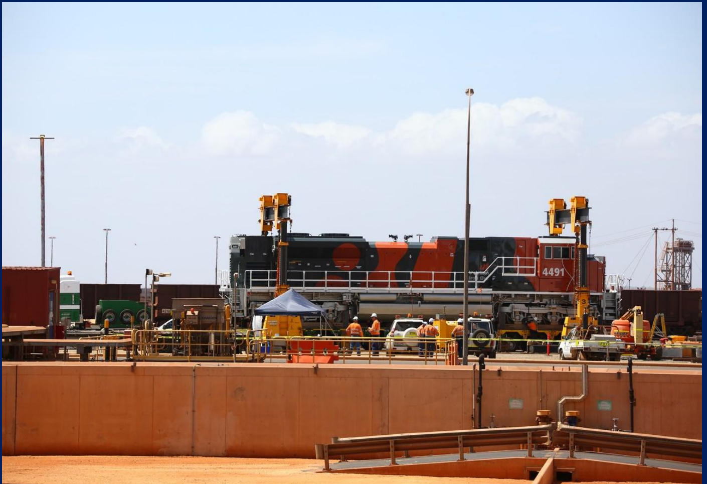
Final SD70ACe 4491 being lifted off transport float by jacks at Nelson Point 16/1. Photo Toad Montgomery
