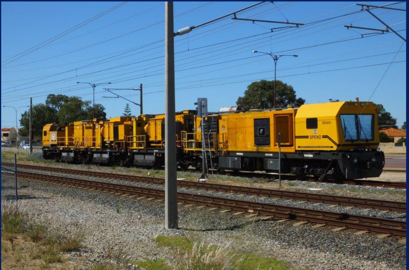
PTA ex Rail Maintenance New Zealand Speno RR24M30 rail grinder in Cannington siding 24/1. Photo Jim B
