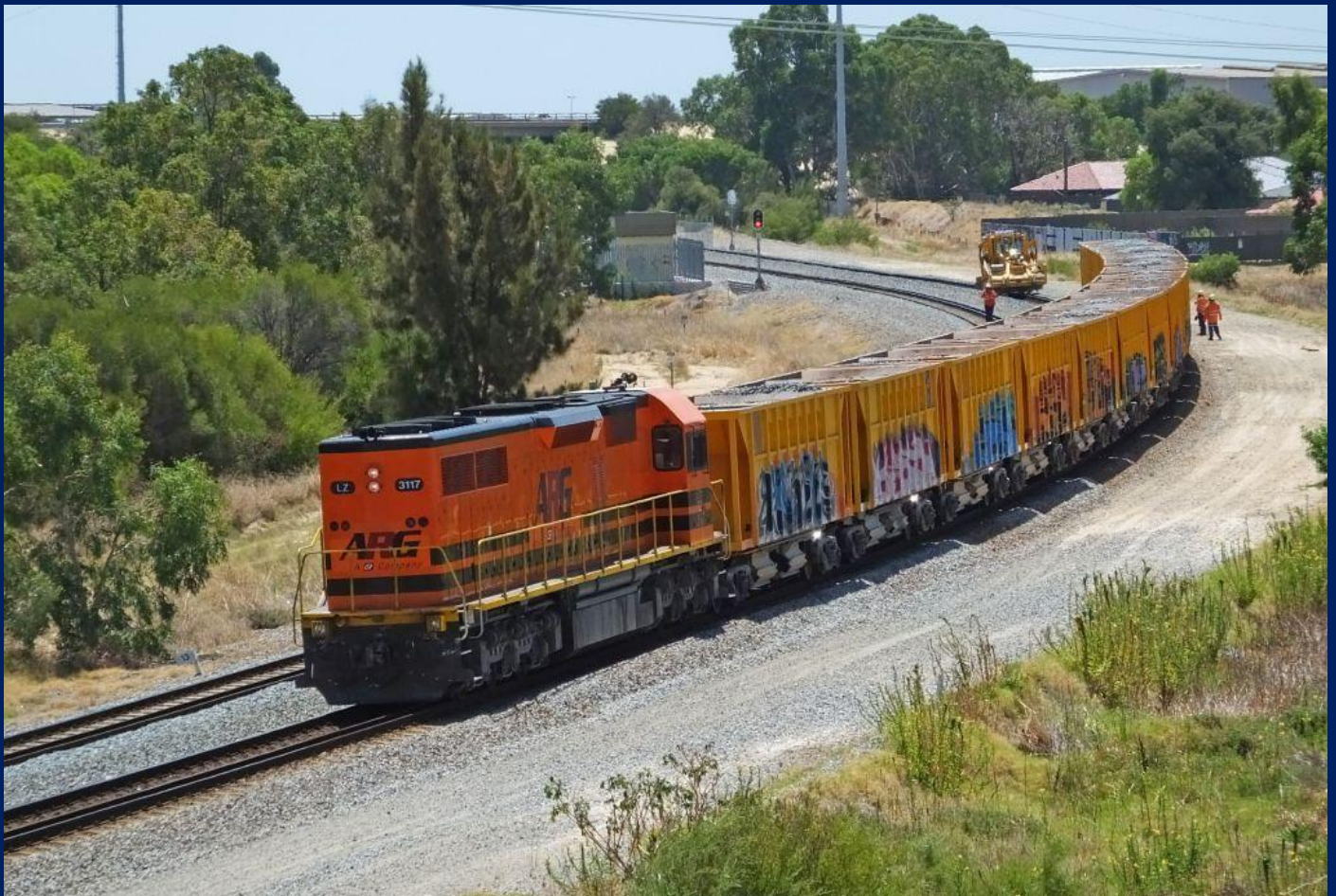
LZ3117 on 4BT2 spot ballasting at Forrestfield south with ballast regulator 17/2.
