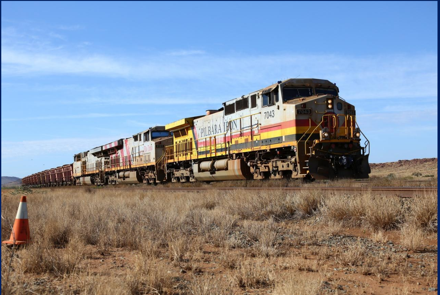
7043, 8131 & 8114 on loaded ore Dingo Siding note the auto haul sensors above the ditch lights March 5th.
