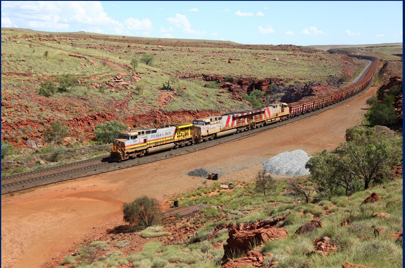
9-CW44 7054 & ES44DCi 8192 & 8163 on loaded ore descending the grade in dynamic brake on March 5th.
