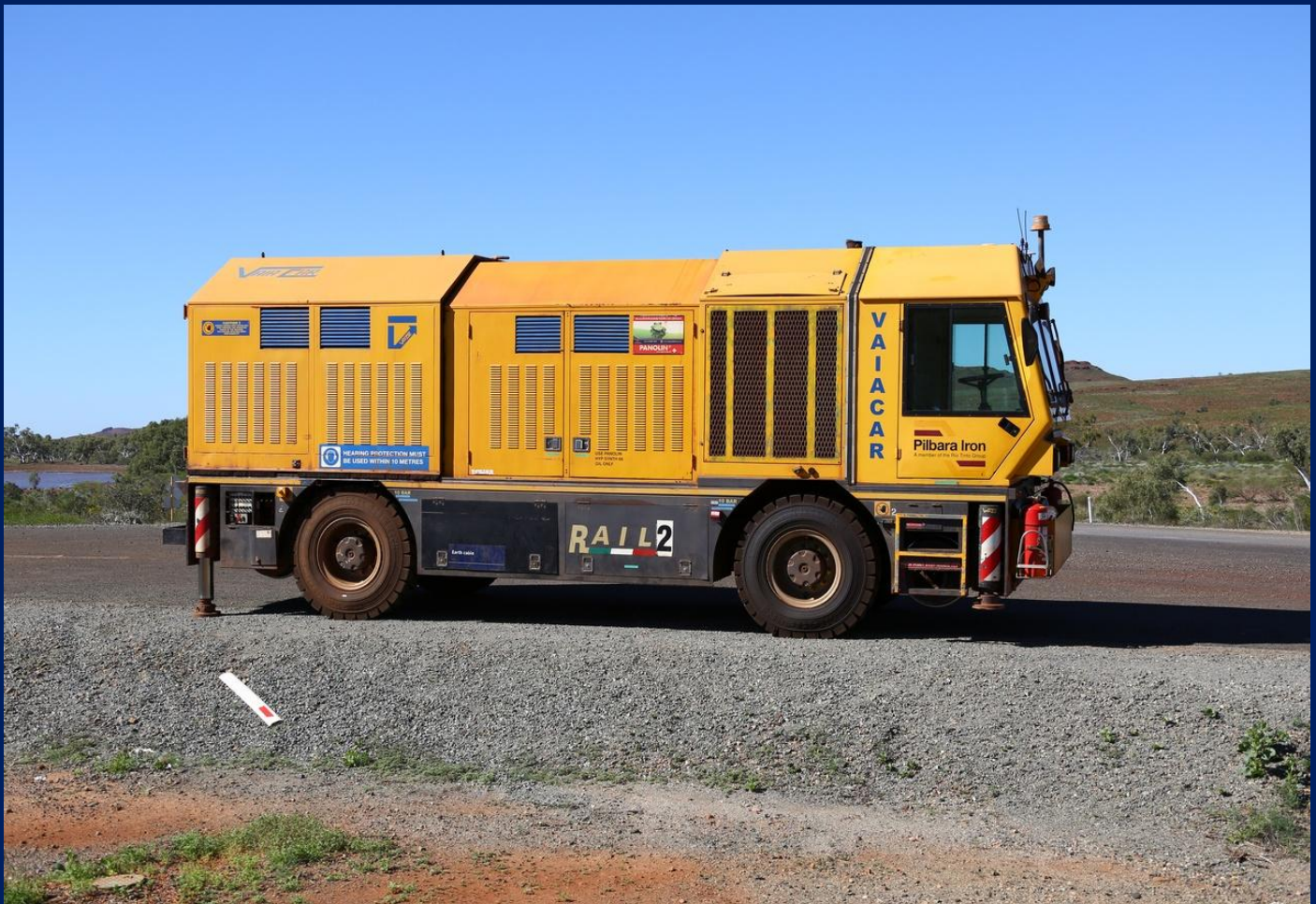
Pilbara Iron mobile flashbutt welding truck Millstream July 27th.
