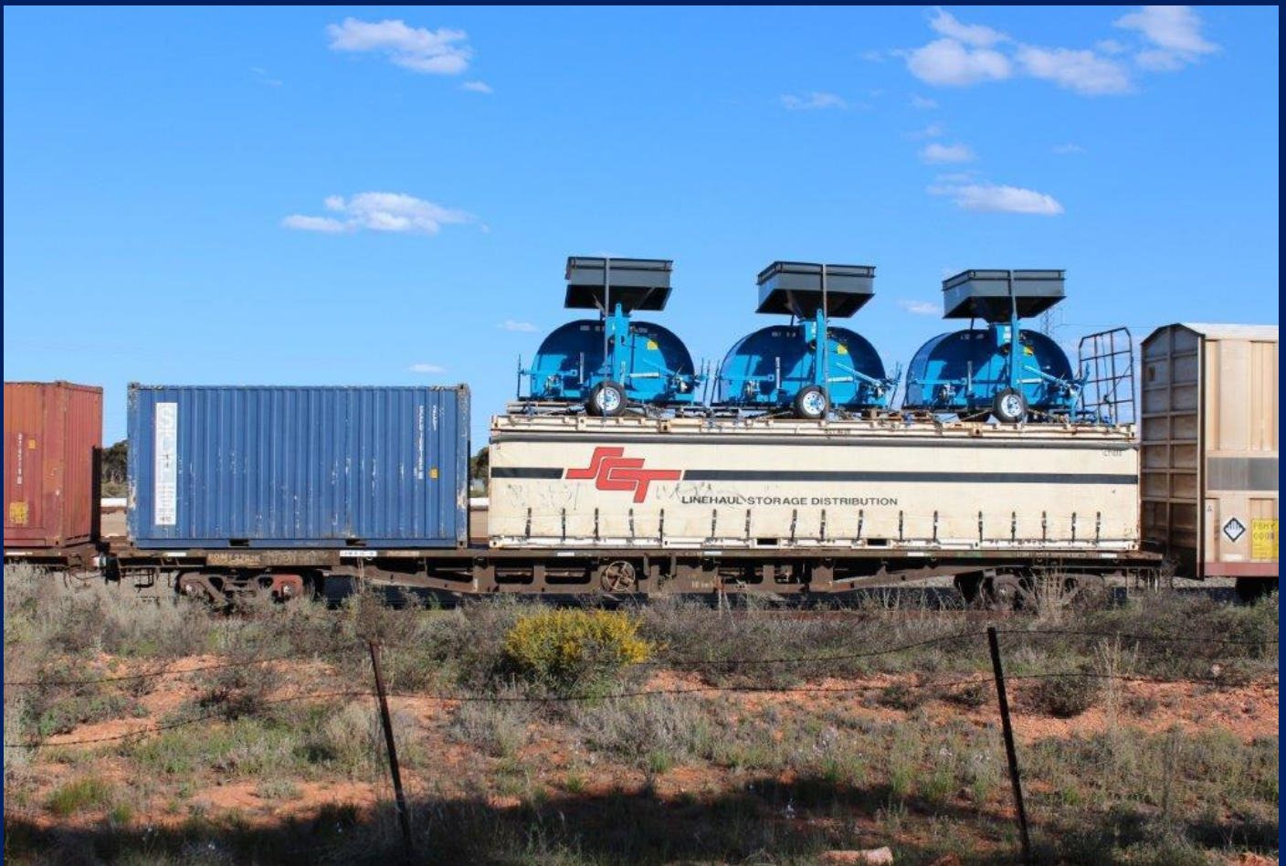
ISO 20 foot container, low profile curtain sided container, double stacked SCT freight. Photo Peter Donaghy
